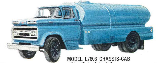
MODEL L7603 CHASSIS-CAB with milk tank body*
