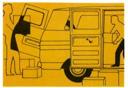
LOADS FROM THE SIDE AND REAR through big double doors that open to either 100° or 180° position. Double doors are also available for left side\* to permit streetside loading as well.
