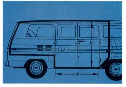
**OVER 175 CU. FT. OF CARGO SPACE** with convenient loading height all the way around. At side doors, load floor is less than 14 inches from ground; at the rear it's less than 27 inches—as low and convenient as the platform of many station wagons.
