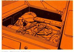
**REAR ENGINE DESIGN.** 80-h.p. air-cooled Turbo-Air 6 engine is capable of greater over-all economy than conventional engines. Its location over the drive wheels, plus 4-wheel independent suspension, assures superior traction and handling, even in sand, snow, or off the road.
