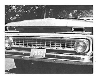
The new Custom Grille is made of corrosionresistant silver-anodized aluminum. Neither weather nor wear can affect its beauty and durability.
