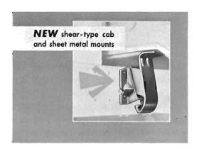
For more comfort, Chevrolet Trucks are first in the industry with new shear-type rear cab and front sheet metal mounts which cushion the cab and driver from fatiguing and destructive vibrations. On E80 Diesels, cab improvements include the addition of 20 body reinforcements, plus new shackle-type rear cab mounts and a flexible hood panel mounting.
