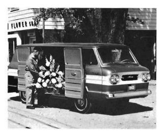
The Corvan has wide, low doors for easy loading and unloading. Left-hand doors are available for operations in crowded areas. Loading doors have new, strap-type, two-position door checks. Optional equipment for Corvans includes rear-door windows.
