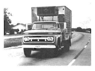
Radiator shutters are available as an option for D60 models this year.\* They keep engine temperatures in the most efficient range under a wide variety of operating conditions.
