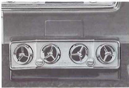
Chevelle Custom De Luxe Air Conditioner and Controls (RPO C65)
