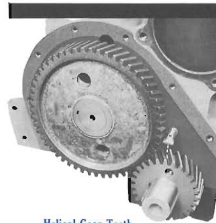
Helical Gear Teeth
