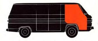
choice of seats-Single driver's seat is standard. Single seat offers extra load space up front, where packages can be stored within easy reach. Fullwidth (3-man) front seat is available at extra cost.
