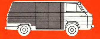
191 cubic feet of cargo space-Corvans carry bigger cargoes-nearly two-thirds of the length is load space! Load compartment is 53.7" high, 120.9" long and 58.6" wide . . . every inch is accessible from the driver's compartment!
