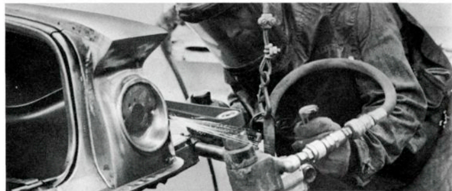
Grinding smooths the body before painting.
