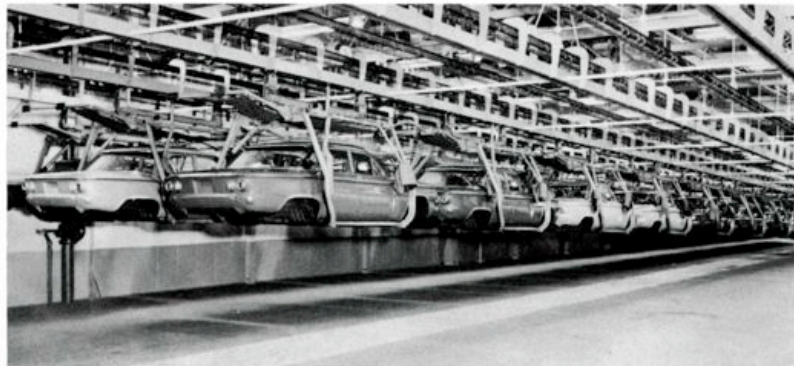
Corvaire bodies come from the adjacent Fisher Body plant in cradles which move slowly on monorail system.
