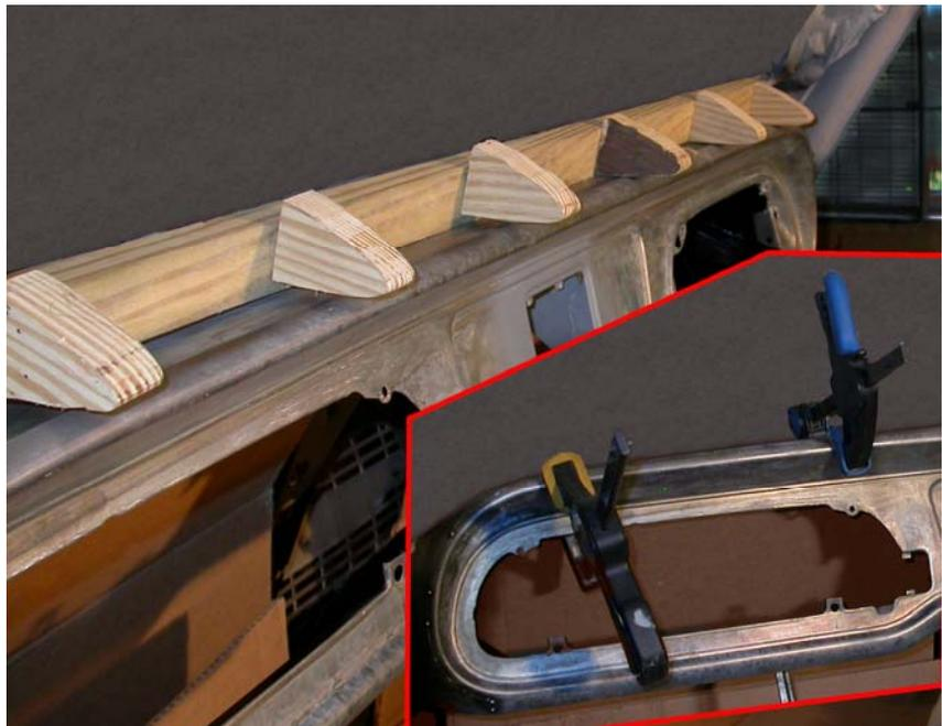
Assorted clamps to the window posts, etc. were used to align the edges (Figure 7). With the accurate cuts, alignment was not difficult to achieve.
