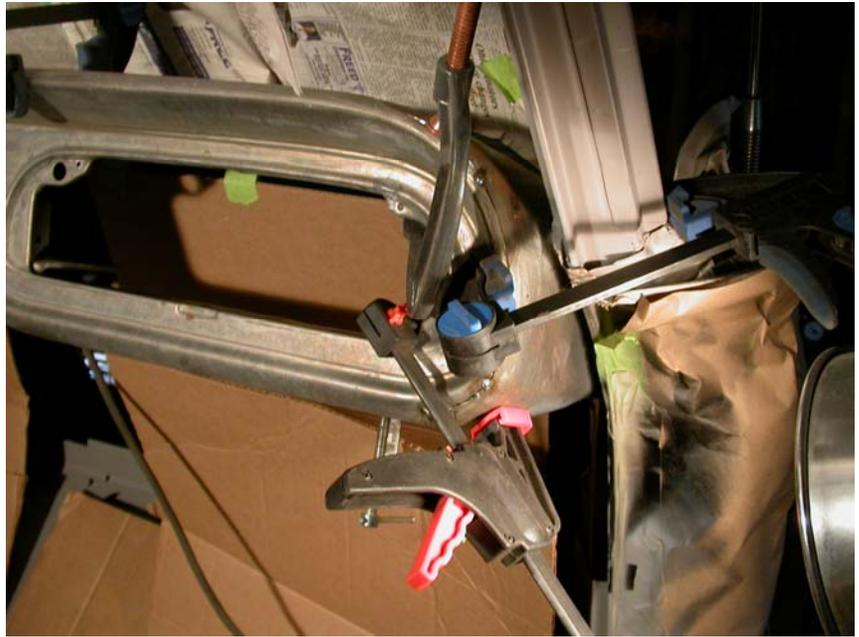
The rest of the story is pretty routine. The edges received a continuous weld and the top was spot welded about every half inch (Figure 8; probably overkill). The dash was plug-welded at the bottom onto the support brackets.
