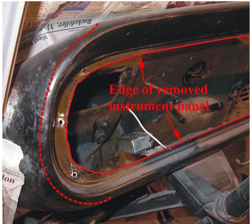
I decided it would be easier to refinish the inside of the old and replacement dashes prior to installation. The fourth figure shows the original dash after the front was removed and the underside was stripped, primed and painted. The weld seam was refinished afterwards.
