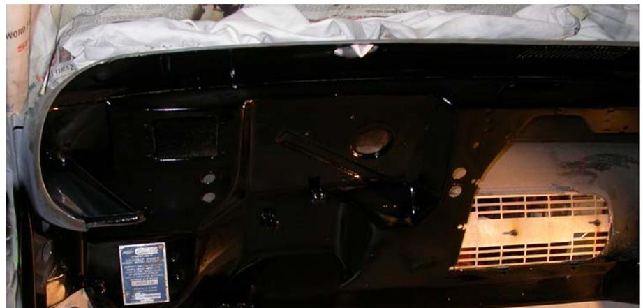
I had discussed the project with a local body shop, and they suggested that the new dash could be simply slid over the old metal to form the lap joint, and this may have worked but I worried about reestablishing the surface profile. I decided instead to flange the edge of the old dash. I made a flanger by welding 18g steel tabs to a welding c-clamp (fifth figure). When clamped tightly to the cut edge of the old dash and hammered laterally along the edge, a perfect flange was produced.
