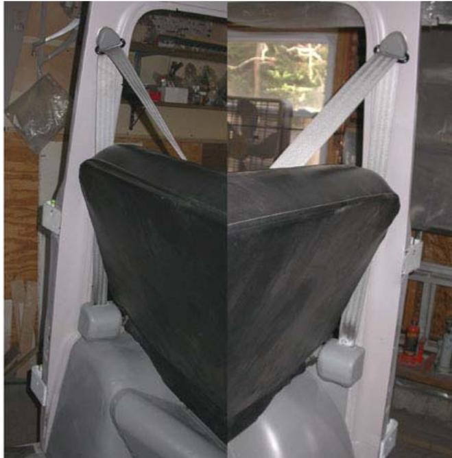
This shows the positions of the buckle ends. The bolt holes are about 3½” off center.
