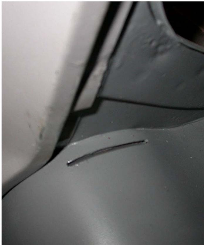
Here is a view under the left wheel well, where the seat belt bracket will connect. The ½” bolt hole through the body strut can be drilled through the gas tank filler tube hole. Removal of the gas tank filler tube is necessary.
