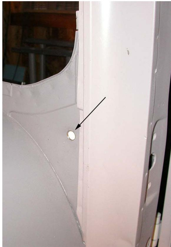
Here is a view from inside the right side wheel well with the retractor bolted through the 1/4" reinforcement plate, which was plug welded in place.
