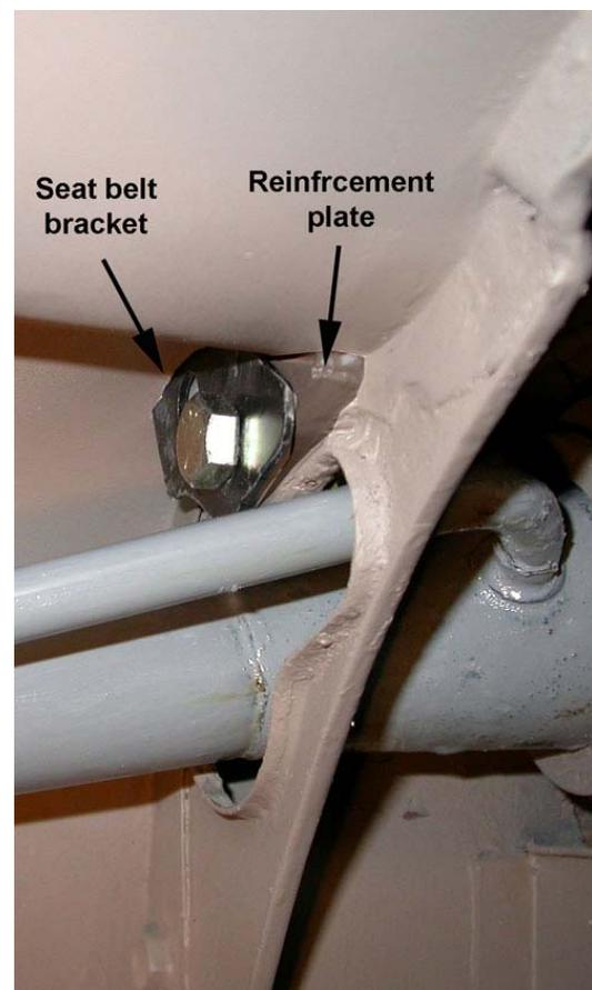
Here is the position of the hole for the right side retractor.
