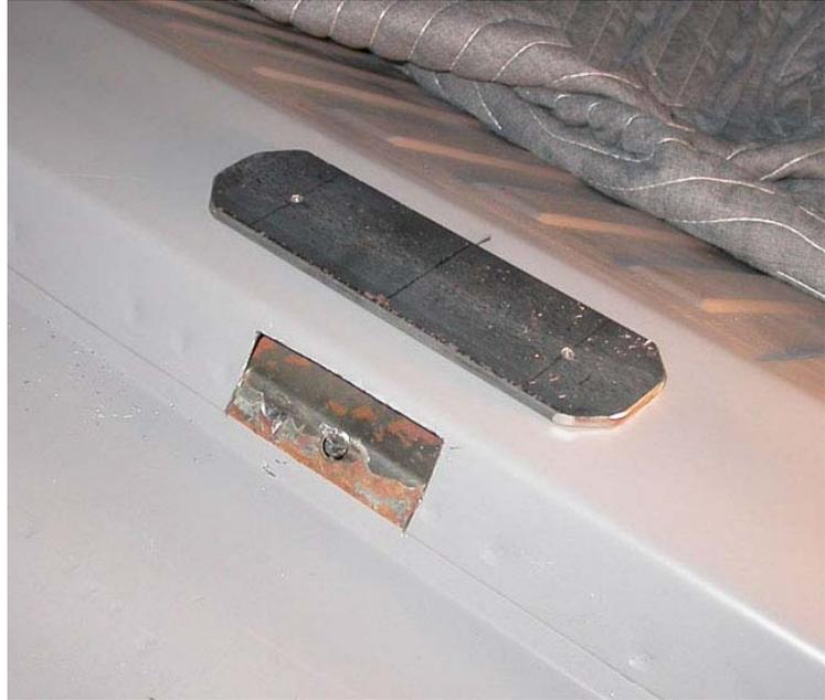
An improvised spatula was used to guide the reinforcement plate into position (very easy), and then the plate was temporarily bolted so that it could be plug welded into place.
