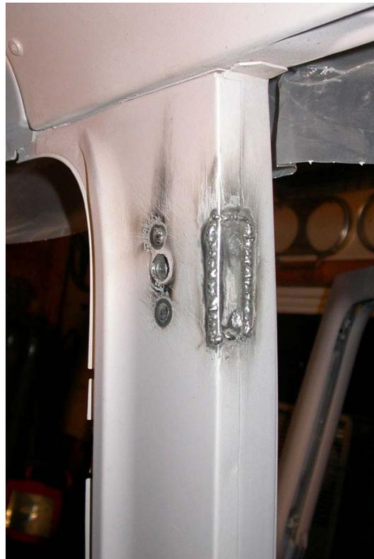
The buckle end belts bolt through a  $\frac{1}{4}$ " reinforcement plate placed in the bulkhead under the seat. The 7" x 2" reinforcement plate is shown here. A small access hole was cut in the front of the bulkhead. Two spot welds had to be removed. To assure proper alignment,  $\frac{1}{8}$ " pilot holes in the plate were used to drill matching pilot holes in the bulkhead; and then expanded to  $\frac{1}{2}$ " diameter. Nuts were welded on back side of the reinforcement plate.
