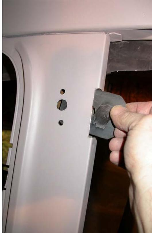
The plate was temporarily bolted and then plug-welded in place. By using the thin cut off wheels, the removed metal can be welded back in place and refinished.
