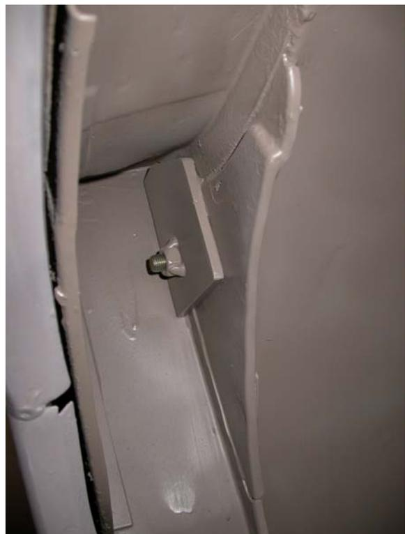
This shows installation of the ¼” reinforcement plates for the door post pivots. Using Dremel 409 cut-off wheels, the body skin and interior metal were cut away to allow inserting the reinforcement plate, which has the nut welded on the back side. The bolt hole must be drilled through the interior metal panel to allow the bolt to fully screw in.
