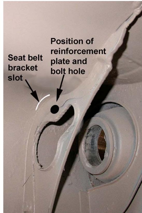
This shows the bracket bolted through the reinforcement plate and body strut. By adding an additional ½” steel, the left side retractor reinforcement plate was made ¾” to completely fill the gap between the seat belt bracket and the wheel-well strut to which it was bolted. The reinforcement plate was plug welded in place. The bracket hole is sealed with a little silicon sealer.
