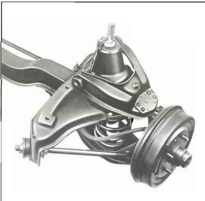
Fig. 4-7—Corvair Lower Control Arm and Strut
