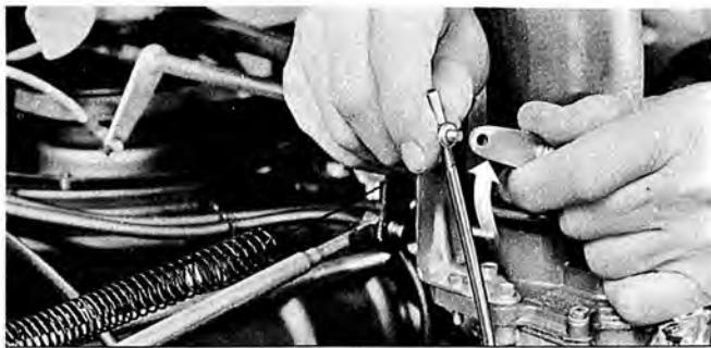
Connect right carburetor linkage to cross shaft. Then, make sure cross shaft is fully turned clockwise, and lift left throttle rod and adjust swivel so it just passes through hole in cross shaft lever. Throttle action will then be synchronized.
