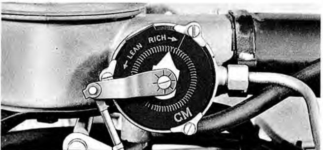
Adjustment of the automatic choke is at the choke modifier. Normal setting is 3-notches lean. To adjust, loosen screw holding lever and pointer, and move pointer counterclockwise 3-notches lean and tighten screw, holding adjustment in position.
