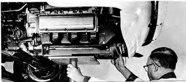
If necessary to perform major overhaul work on any of the power components, removal and replacement of the power train package involves only a few procedures, and takes less than 2 hours. Follow Section 6-4 of the Corvair Shop Manual for a step-by-step listing of the necessary procedures.
