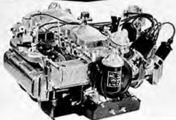
Construction details of the air-cooled Corvair engine are unique in many respects, but basically require very few additional service procedures than you're accustomed to.
