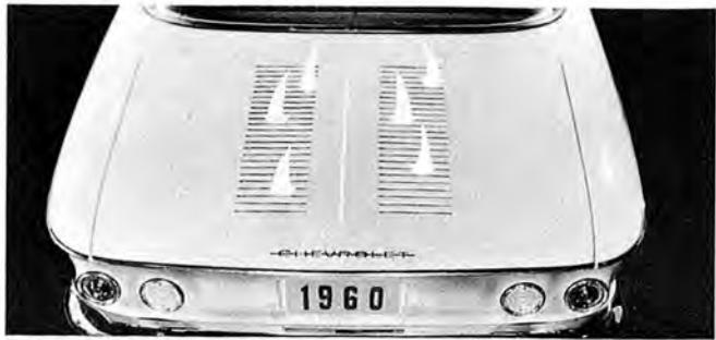
Air for cooling and carburetion is drawn through louvered deck lid. There is no danger of engine overheating if lid is snow- or ice-covered, but sluggish performance will result. The blower will exhaust almost all available air in the compartment, leaving an insufficient amount for combustion.
