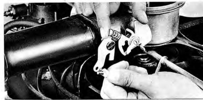
Hold the screw and fast-idle lever in position and turn the swivel on the fast-idle link so it just enters hole in the fast-idle lever. Replace retainer clip and remove the  $\frac{1}{8}$ " spacer. Trim adjusting fast-idle screw to obtain a speed of 2200 r.p.m.
