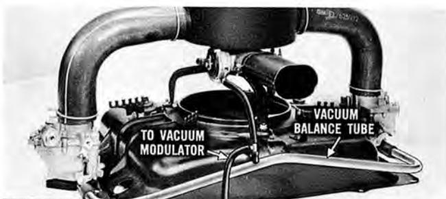
These model "H" downdraft carburetors are interchangeable, left or right. A vacuum balance tube connects the two intake systems to improve idling smoothness, and to provide vacuum from all six cylinders to help operate automatic choke and vacuum modulator on Powerglide cars.
