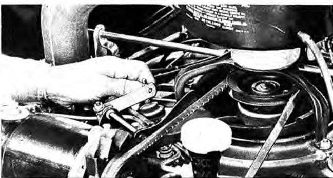
Next, disengage swivel from hinge lever. Then, holding air control valve open  $1\frac{1}{2}$ ", adjust swivel so it just enters hole in hinge lever. Replace retainer. Don't bend hinge or bracket to correct valve height.
