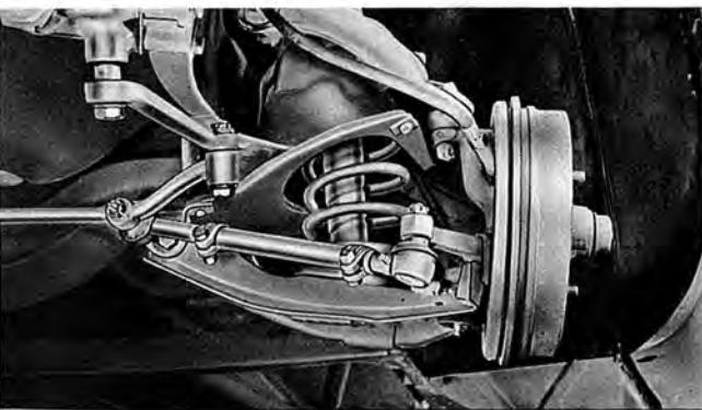
Front suspension alignment follows conventional procedures. Make all adjustments with luggage compartment empty, except for spare wheel.
