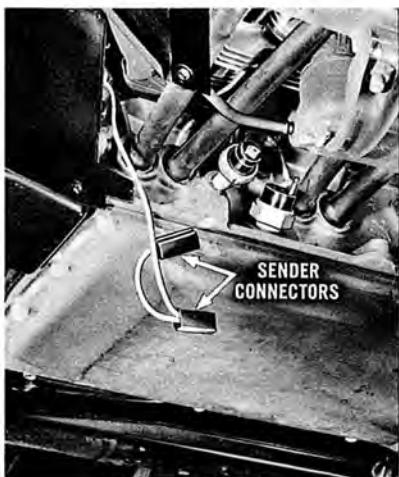
Check for grounded sender circuit by removing sender connectors. Turn ignition to "ON." If light comes on, circuit is grounded. (Shrouding is removed for photographing purposes.)
