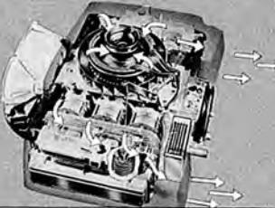
Forced air from a belt-driven blower is directed around the engine by a metal shroud. The size and speed of the blower and the design and routing of the shroud are carefully calculated to cool engine at all speeds.
