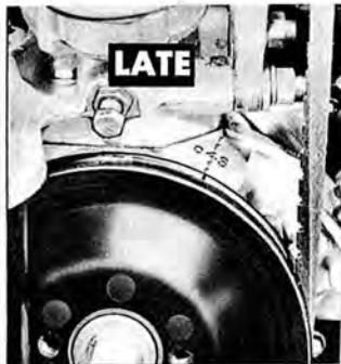
First production engines used the markings "O" and "A" on timing pointer tab. This was later changed to degree marks "0-4-8." Time early engines  $\frac{1}{2}$  the distance from "O" to "A." Late engines are timed 4 degrees BTDC.
