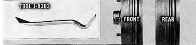
Tool J-8363 is required for brake adjustment as follows:
