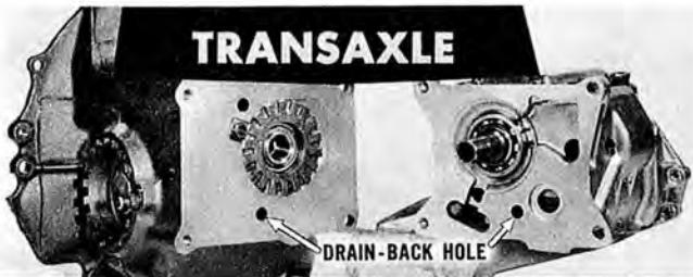
Three-speed Transaxles have a common oil supply. The transmission receives throw-off oil from the ring gear. A drain-back hole is located above the safe operating level of transmission, so a quantity of lubricant is retained. For routine 1,000-mile inspections, check level at differential. If oil is up, transmission will also have an operating supply.
