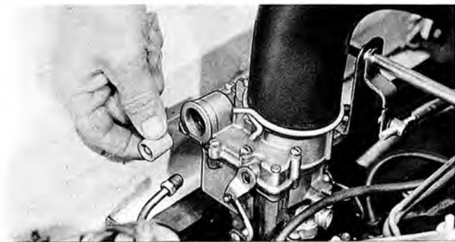
Both carburetors contain a sintered bronze inlet gasoline filter like other Chevrolet carburetors. Filters should be cleaned every 5,000 miles and replaced at 15,000-mile intervals.
