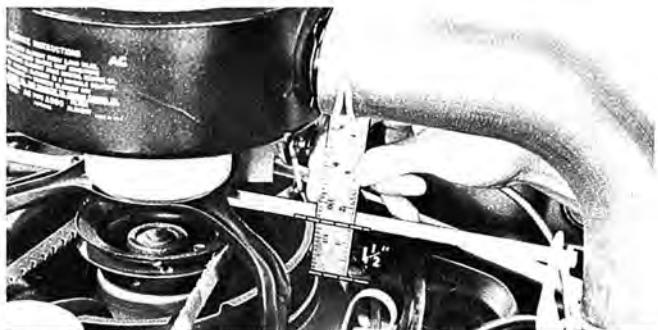
To check air control valve for proper clearance, bring engine to operating temperature. Then, pull up on push rod from thermostat to its upward limit. Valve should be open  $1\frac{1}{2}'' \pm \frac{1}{16}''$  measuring at a point opposite hinge as shown here.
