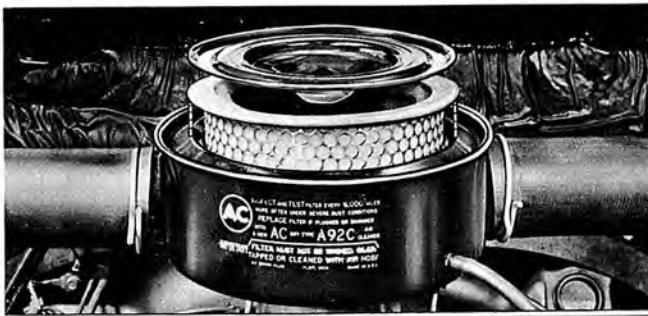
Place element in air cleaner body. It should be allowed to drop lightly into position so the upper flared lip extends outside the top of the air cleaner. Next, install cover over center stud and tighten so lid will "crush" edges of element against cleaner body, thus forming a seal.
