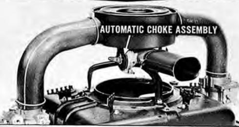
Each cylinder head has an integral intake manifold and is provided with its own carburetor. Both carburetors receive air through a common air cleaner and automatic choke assembly.
