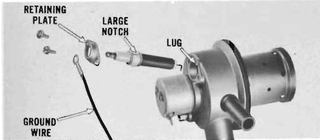
Install spark plug with gaskets and rubber sleeve in burner housing. The large notch in the spark plug porcelain indexes with a lug in the burner housing to provide correct electrode alignment. Ground wire should be installed between attaching screw and retaining plate as shown.
