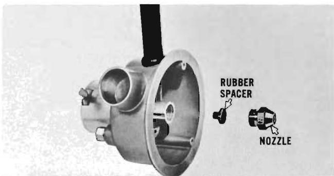
If the cause of fuel blockage is not due to an inoperative solenoid, all other components of the fuel section should be removed and inspected. Remove fuel nozzle and rubber spacer.
