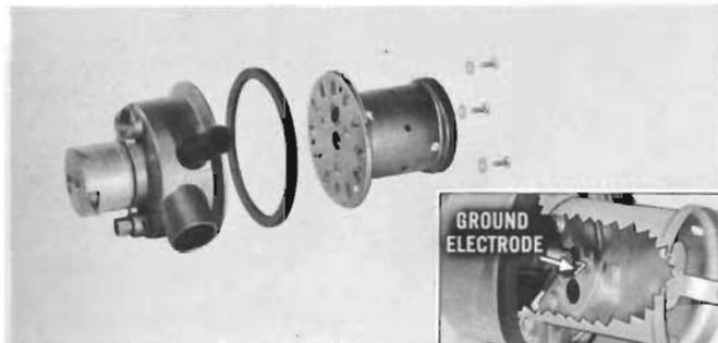
If mixer cup must be removed because of a badly burned shell, a burned-away ground electrode, or to test or service the fuel section of the burner housing, remove three screws which secure cup to housing. Separate mixer cup and gasket from housing.
