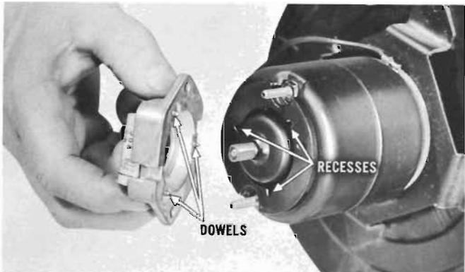
Install new ignition unit making sure the three locating dowels enter the recesses in motor end plate.
