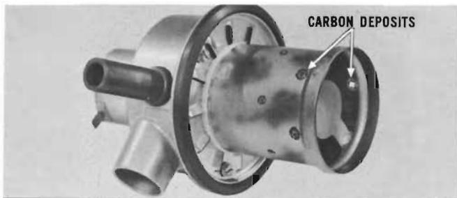
If the carbon build-up is uneven, carbon deposits clog or partially clog the air holes, or small areas of the mixer cup are excessively burned, the burner has been operating with an insufficient supply of combustion air, a one-sided fuel spray; or there has been fuel leakage inside burner casting.
