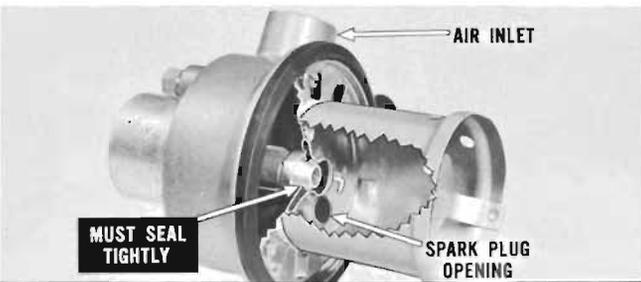
Install mixer cup and gasket, aligning spark plug openings in mixer cup and burner housing. The full circumference of the center opening in the mixer cup **MUST** seal firmly against the tapered end of the fuel nozzle. Check by looking through air inlet. There should be no light visible around nozzle.
