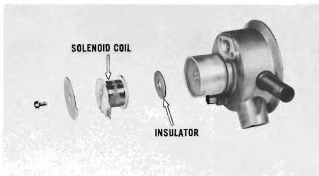
Remove solenoid coil cover screw and cover. Install new solenoid coil. Make sure insulator between solenoid and solenoid cup is in good condition.
