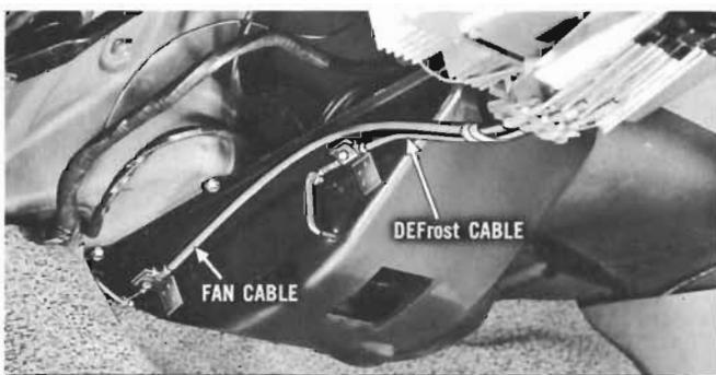
The DEFrost and FAN control cables have "eyed" ends at air distributor. The only adjustment possible to obtain full travel of either of these controls is by shifting the cable sheath in its retaining clamps.
