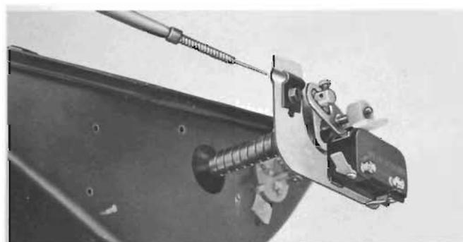
Disconnect HEAT control cable from thermostat and remove screws which secure thermostat to air distributor. Install new thermostat and adjust cable as shown previously.
