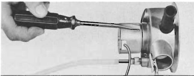
If no fuel sprays from nozzle, the solenoid coil, fuel inlet screen, fuel valve or nozzle assembly could be at fault. Check the solenoid coil by opening and closing the solenoid electrical circuit while holding the blade of a screw driver close to the solenoid cup. A good coil will attract the blade when the coil is energized. If solenoid coil is not functioning, stop engine and replace coil as follows:
