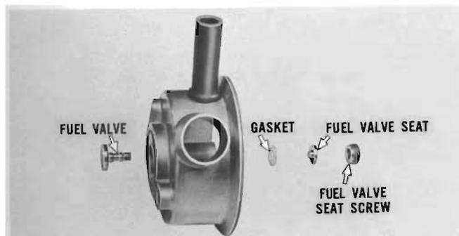
NOTE: It is not normally necessary to remove the fuel valve seat screw, valve seat and gasket from the burner housing. If these parts are removed for any reason, the fuel valve nylon gasket must be replaced.
