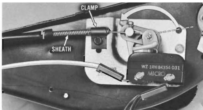
Move HEAT control lever to full "up" position. Make sure there is no interference with cable sheath when thermostat tension lever is in full counterclockwise position.
