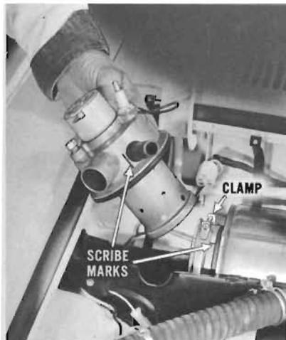
Scribe a line across burner and heat exchanger. Loosen burner clamp and pull burner out of heat exchanger and place on bench.
