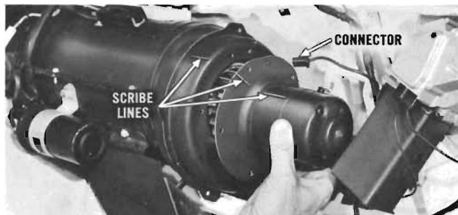
**VENTILATOR BLOWER:** To remove ventilator blower from heater, separate connector at motor terminal. Scribe a line across blower housing, motor mounting plate, and motor. Remove four retaining screws and remove motor and fan assembly.
