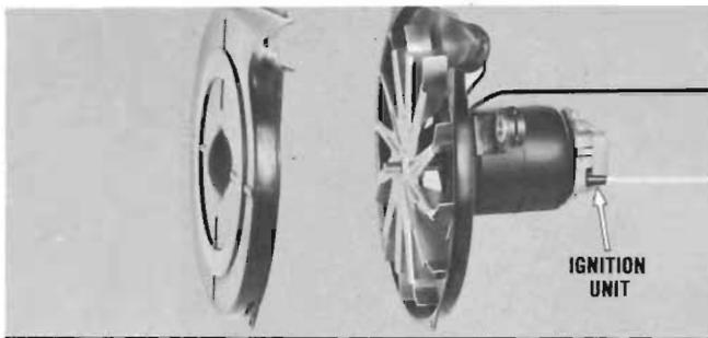
Locate fan on shaft so blades clear inner case. Tighten Allen screw. Attach outer half out of case to inner half. Install cam and primary ignition unit on end of motor. Check ignition point gap as shown earlier. Install blower assembly on car.
