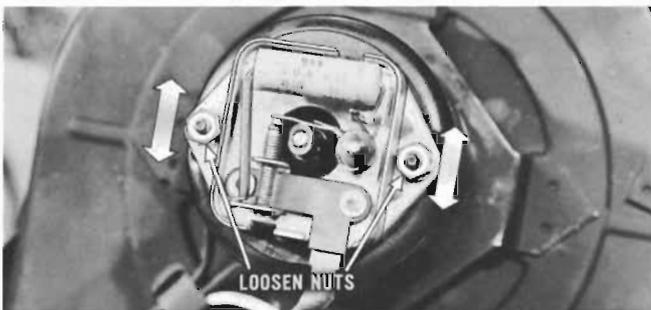
If point gap readings are within .010" of each other but either is below .012" or over .021", try to bring both gaps within desired reading by loosening the two ignition unit mounting nuts and shifting assembly slightly as permitted by bolt hole clearance.
