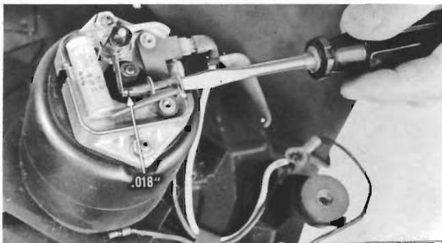
Adjust new points by turning threaded stationary point until gap on each lobe is approximately midway between .012" and .021". (Preferable gap is .018" on each lobe.)
