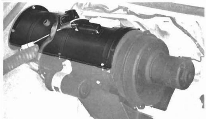
**BURNER ASSEMBLY:** To get to the burner assembly, the top half of the heater case must be removed as follows:
