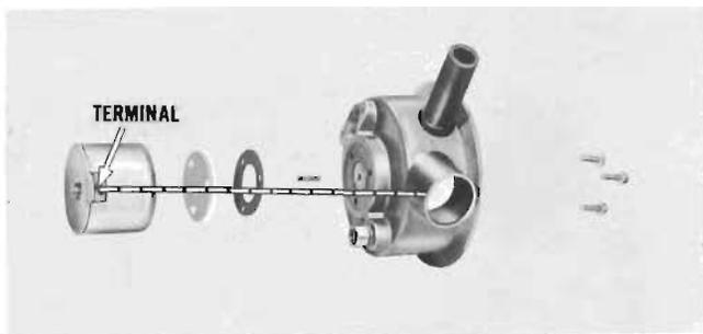
**NOTE:** When installing solenoid cup assembly, use a new gasket between sealing disc and burner housing. Make sure coil terminal is approximately in line with burner air inlet opening. Retest burner assembly for correct spray pattern and complete fuel shut-off.
