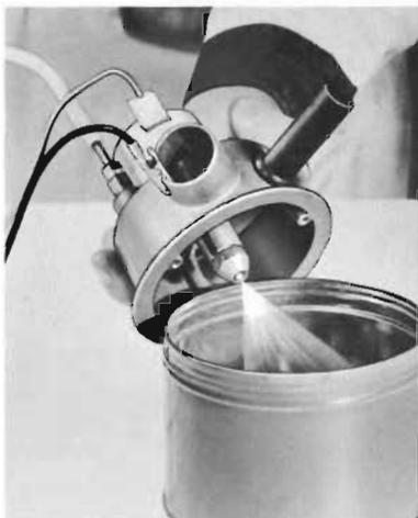
Have someone start engine and connect electrical lead from solenoid to a live terminal on the car (red wire at horn relay, or brown wire at windshield wiper connector). Fuel should spray uniformly from nozzle.
