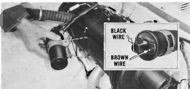
**COIL:** When replacing coil be sure brown wire is connected to the primary negative (-) terminal and the black wire connected to the primary positive (+) terminal. **NOTE:** This is a special high voltage coil. Do not attempt to replace it with a standard automotive coil.
