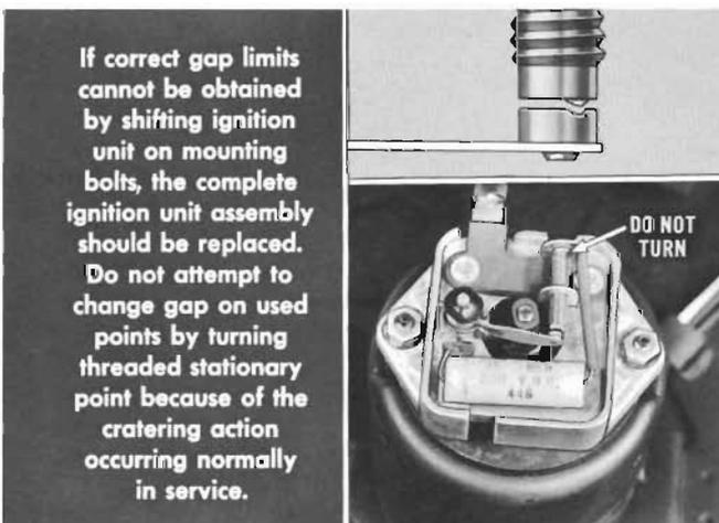
If correct gap limits cannot be obtained by shifting ignition unit on mounting bolts, the complete ignition unit assembly should be replaced. Do not attempt to change gap on used points by turning threaded stationary point because of the cratering action occurring normally in service.
