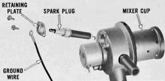
Remove two screws which secure the spark plug retaining plate and ground wire to the burner housing. Remove spark plug. Inspect spark plug electrode, and the ground electrode attached inside the mixer cup. If electrodes are badly burned, both the spark plug and the mixer cup must be replaced.
