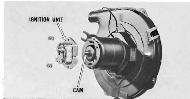
If points are damaged, if there is evidence of condenser failure, or cam is excessively worn — disconnect primary lead, remove two nuts and lockwashers, and remove ignition unit.
