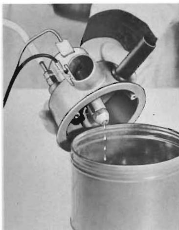
Have someone disconnect live electrical lead at car. Fuel spray should stop. NOTE: A momentary dribble of fuel from nozzle is normal. There should not be a continuous dribble.
