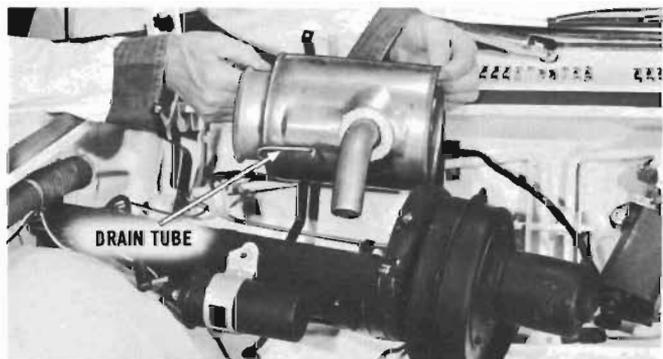
Disconnect the drain hose from the heat exchanger drain tube. Shift the lower heater case towards the front of the car. Remove heat exchanger.
