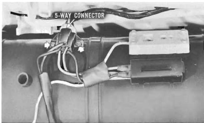
Loosen 5-way connector attaching screws. Slide connector loose from case. Separate connector.
