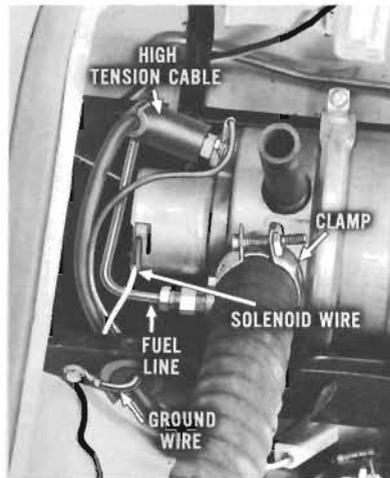
Remove the burner assembly from the car as follows: Disconnect the spark plug ground wire and fuel solenoid wire. Separate high tension cable from spark plug. Disconnect fuel line to burner. Loosen clamp securing combustion blower hose to casting.
