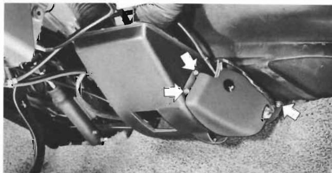
**HEATER CONTROLS:** The adjustment of the HEAT control cable is very important. To check adjustment, remove screws from cover on right side of air distributor. Remove cover.
