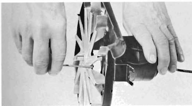
Remove ignition unit from end of motor as shown earlier. Remove outer half of blower case and loosen Allen head screw in inner side of fan hub. Pull fan off shaft.
