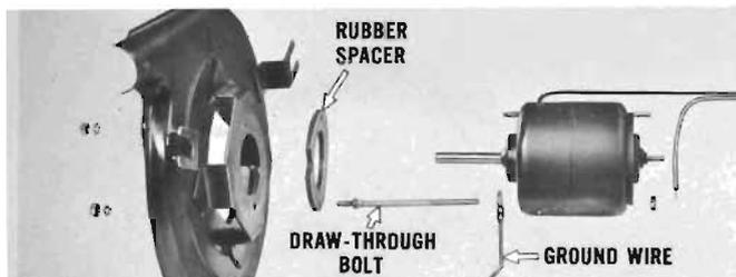
Remove the two nuts and lockwashers from the inner half of the blower case. Separate motor and rubber spacer. When reassembling, attach the ground wire between the draw-through bolt and the motor housing. **NOTE:** Replacement motors have two wires. The black wire leads into the motor case. The white wire is an extra ignition unit wire and should be discarded.
