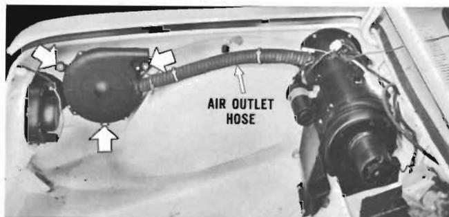
**PRIMARY IGNITION UNIT:** The primary ignition unit can be serviced without removing the combustion blower entirely from the car. Disconnect the outlet air hose and remove the three bolts which secure the combustion blower assembly to the fender.
