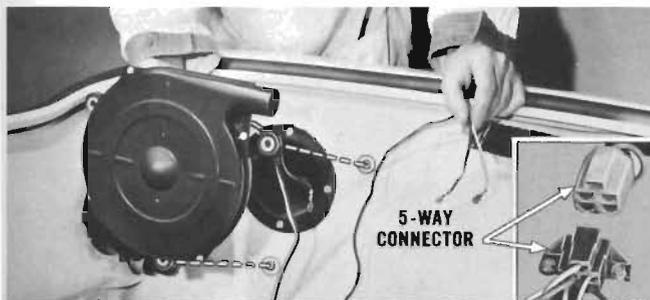
**COMBUSTION BLOWER:** Separate 5-way connector located on heater. Remove black and white wires leading to blower from the connector. Free these wires from clips. Disconnect outlet hose from blower. Remove the three attaching bolts and remove blower from car.
