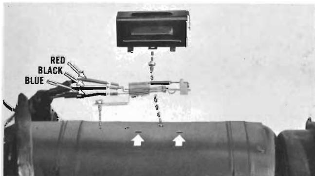
When replacing Purge Switch, be sure to solder wires to new switch as shown. Note that switch cover is secured by two spring tangs in front and one screw at rear.
