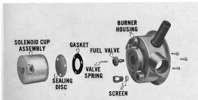
Remove fuel inlet fitting and screen. Remove three screws securing solenoid cup assembly to burner housing. Separate solenoid cup assembly, sealing disc, gasket, fuel valve spring and fuel valve from burner housing.
