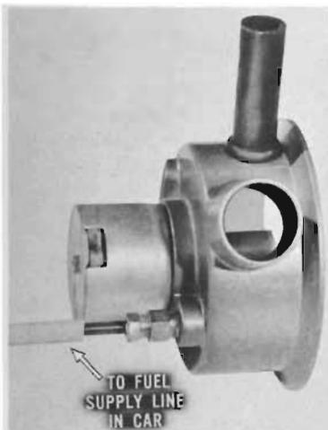
Connect a hose from the heater fuel supply line in the luggage compartment to a short piece of pipe installed in the burner housing fuel inlet fitting. The hose should be long enough so the burner housing can be located outside the luggage compartment.
