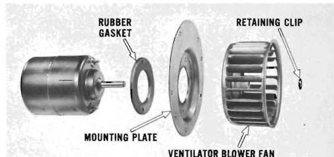
To remove fan, loosen retaining clip (or set screw) which ever is used. Install new blower motor or fan as required. Reverse procedures to assemble and install. (Use the alignment marks to assist in proper reassembly and installation.)
