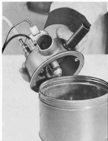
Run a lead from the fuel solenoid terminal to some point where it can be connected to a convenient live terminal on the car. (Do not connect lead at this time.) Connect a ground lead between the car and the burner housing. The electrical lead should be connected and disconnected at the car because of the hazard of arcing at the burner assembly and possible ignition of gasoline.
