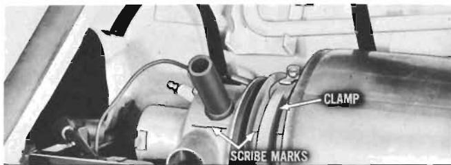
Install burner assembly so scribe marks on burner assembly and heat exchanger are aligned. Connect fuel line to burner housing fitting before installing retaining clamp. Tighten clamp securely. Before connecting fuel solenoid wire and installing upper half of heater case, start engine and check for fuel leaks. Complete the assembly of the heater following the removal procedure.
