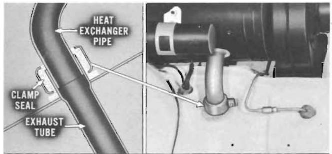
Install the heater exhaust tube, making sure it projects up into the luggage compartment. This locates the heat exchanger pipe correctly inside the exhaust tube, and the clamp and clamp gasket can now provide a good seal. Tighten the clamp securely. Install the metal shield.
