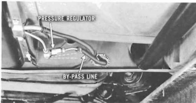
**PRESSURE REGULATOR:** When installing a new pressure regulator make certain the by-pass line is at or slightly above horizontal, so air bubbles or vapor will vent to the fuel tank.
