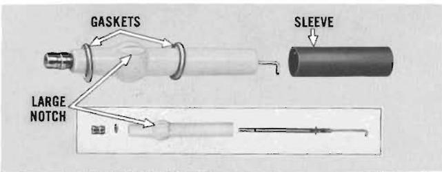
Before installing the spark plug remove the rubber sleeve and carefully inspect the porcelain for cracks. Inspect for badly burned electrode. If necessary, remove the electrode from the porcelain and clean electrode with emery cloth. When reassembling spark plug, the electrode should point away from the large notch in porcelain. Examine rubber sleeve and the two plug gaskets and replace if necessary.
