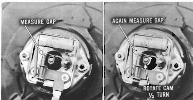
Check for .012" to .021" on each of the two cam lobes. A difference of more than .010" between lobes indicates one lobe of the fiber cam is excessively worn and cam should be replaced as shown later.
