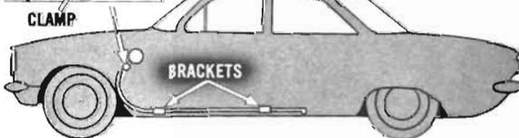
**EXHAUST TUBE:** To replace the exhaust tube, loosen the clamp which secures the exhaust tube to the heat exchanger outlet tube. Remove the bolts which secure the exhaust tube to mounting brackets on the car underbody.
