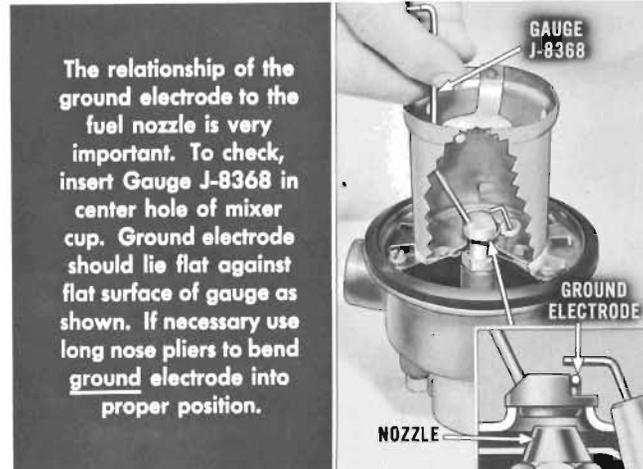
The relationship of the ground electrode to the fuel nozzle is very important. To check, insert Gauge J-8368 in center hole of mixer cup. Ground electrode should lie flat against flat surface of gauge as shown. If necessary use long nose pliers to bend ground electrode into proper position.
