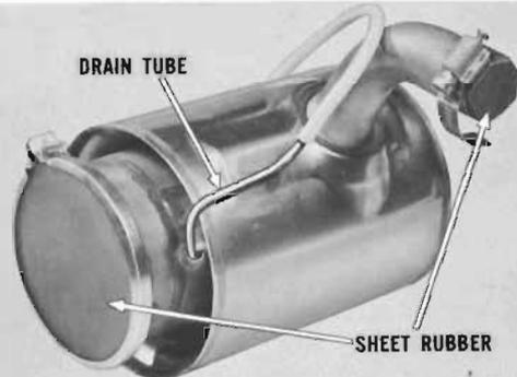
To test heat exchanger, block burner inlet and exhaust outlet openings with sheet rubber held in place with clamps. Connect rubber hose to drain tube.
