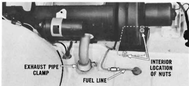
Disconnect exhaust pipe clamp and fuel line connections. To obtain clearance for removing heat exchanger remove two nuts holding ventilator blower case in place. (These two nuts are in the passenger compartment. One is located in the air distributor.)
