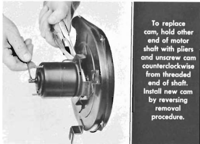
To replace cam, hold other end of motor shaft with pliers and unscrew cam counterclockwise from threaded end of shaft. Install new cam by reversing removal procedure.
