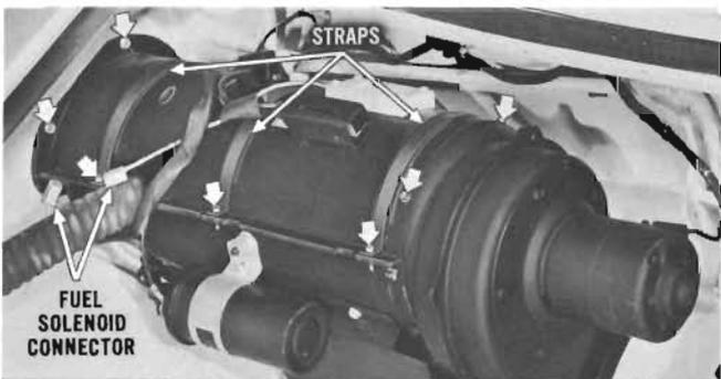
Remove two screws holding upper half of heater case to fender. Remove three strap screws. Remove two top screws holding ventilator blower housing to heater case. Separate fuel solenoid wire connector.
