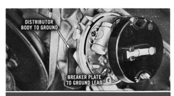
— a poor ground connection between breaker plate and distributor body, or a poor ground at the distributor mounting to the engine. Testing for these conditions requires the use of a meter as follows:
