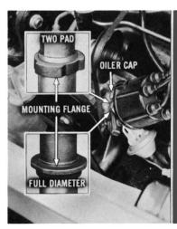
Check the distributor color-coded oiler cap and determine the type of distributor mounting flange used. Two designs are in service, the two-pad type or the full-diameter type. When the oiler cap color and flange design are known, check the following charts to determine the correct specifications.
