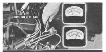
Run the engine at 1500 rpm. Ground the red lead of the secondary resistance tester, then touch each plug (in order) with the black lead. A uniform reading of "5" to "5½" within the GOOD range indicates the secondary circuit components are in good operating condition.
