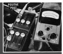
test. Disconnect the positive battery cable from its post and hook up a voltmeter between battery post and cable. All switches and accessories must be OFF.
