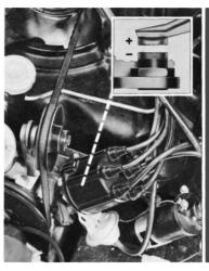
Primary circuit operating voltage over 12.5 volts causes excessive current flow through the points (when closed). This produces excessive heat at the points, which, in turn, results in rapid point burning or bluing. In doing so, an oxide coating forms on the point contact surfaces.
