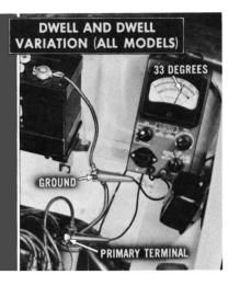
If dwell reading is not within limits, recheck the point gap and, if necessary, regap points to obtain proper dwell specifications. Use a screw driver as shown to make adjustment. Also inspect carefully for a misaligned point rubbing block or a worn distributor cam.
