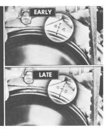
This on-the-car test quickly checks the degrees of spark advance produced by the centrifugal and vacuum control units. Connect a tachometer and advance tester which is equipped with a timing light. Initial timing must be correct to make this check.
