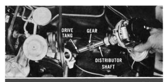
If dwell varies more than the 3-degree limit, pull the distributor (noting rotor position) and check the distributor shaft, the bushings, the breaker plate, gear teeth and drive tang. If any parts are worn or loose, service or replace as required. Repeat dwell tests.
