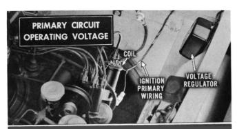
This test is a quick operating check of the voltage regulator, the ignition primary wiring and the coil primary windings. It will also indicate whether short distributor point life is caused by high operating voltage.
