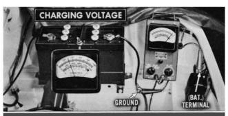
Connect the voltmeter to the battery (BAT.) terminal of the voltage regulator and to a good ground. Run the engine at a constant 1500 rpm. A reading of 14 to 15 volts indicates the charging system and voltage regulator are operating satisfactorily.
