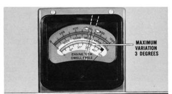
Slowly bring engine up to a constant 1500 rpm. Note the dwell reading. Return engine to idle speed and note the dwell reading again. Dwell reading should not vary more than a total of 3 degrees within the rpm range.
