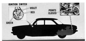
A reading of less than 4.5 volts (points closed) may be caused by loose or corroded wiring at the ignition switch, or main wiring harness connectors, or poor internal contacts in the ignition switch. Inspect all wiring and connectors and correct any electrical difficulty found. If this does not eliminate the cause of low voltage, install a new ignition switch.
