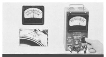
Bring engine rpm up to 2500. Adjust meter knob to electronically align timing mark to proper initial setting. Check the following chart for correct advance specifications.
