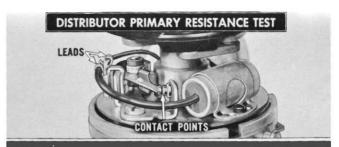
This test measures primary circuit resistance within the distributor assembly. Excessive resistance will reduce primary current flow through the coil, thus weakening its ability to handle peak loads. Factors causing this condition may be traced to oxidized contact points, loose or improperly connected leads, or leads which are frayed internally.
