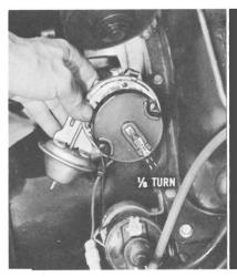
Reinstall distributor by turning rotor about 1/4 turn in a counterclockwise direction past the mark (or noted position) previously made. Mesh gears, install clamp and all connections. Install distributor cap and recheck timing.
