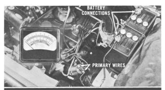
If the pointer reads off the scale to the left with the meter properly connected, it indicates reversed coil polarity. Check for reversed primary wires, battery connections, or battery charged incorrectly. Service as required.
