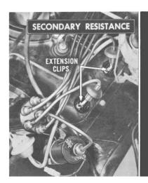
This test checks the ability of the secondary circuit to conduct the proper voltage and current to the spark plugs. Install extension clips between the plug terminals and plug wires.
