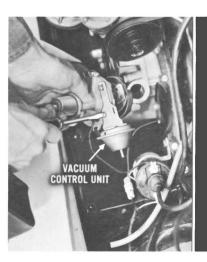
If centrifugal advance now reads correctly within the limits shown on the advance specification chart, the cause of improper total advance is improper vacuum control system operation. If necessary, remove distributor (note rotor position) and install a new control unit. Set advance plate to 23 degrees.
