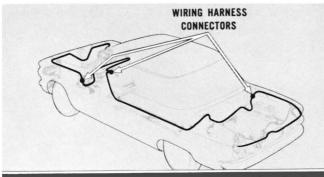
If meter reads a voltage figure, it indicates a short in the wiring or switches. Disconnect each individual wiring harness at the connectors until the voltmeter reads zero, then trace the cause in that particular circuit.
