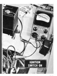
Connect a dwell meter to the primary terminal of the coil, distributor side, and to a good clean ground.
