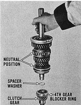
Clamp the mainshaft in a vise with the forward end of the shaft upwards. Remove the special snap ring, the 3-4 synchronizer and 3rd gear blocker ring from the shaft. Remove the 3rd speed gear, the needle-bearing thrust washer, the 2nd-speed gear, and the 2nd gear blocker ring.
