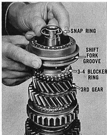
Install the 3rd-speed gear with the clutching teeth upward. Place one of the 3-4 blocker rings on the cone surface of the 3rd-speed gear. Install the 3-4 synchronizer clutch with the shift fork groove downward. Turn the blocker ring until the notches engage the keys. Install the special snap ring.
