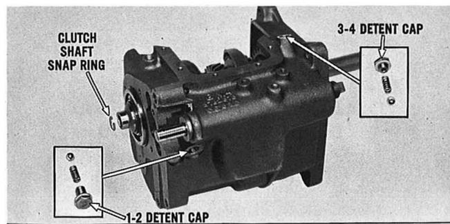
Install both the 1-2 and the 3-4 detent balls, springs, nylon washers and detent caps. The 1-2 cap has the longer thread length. Install the small snap ring in the inner diameter of the clutch gear. This snap ring is a bottoming stop for the clutch shaft.
