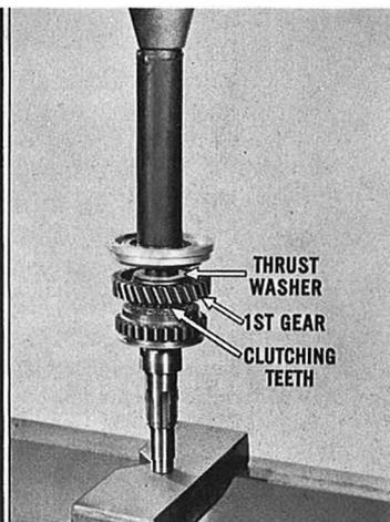
**Mainshaft:** Place the forward end of the mainshaft downward on a press plate. Place the 1-2 synchronizer assembly over the mainshaft with the shift fork groove down. Press the 1st-speed gear sleeve on the mainshaft until it bottoms, using Tool J-5590 or any other suitable hollow driver.
