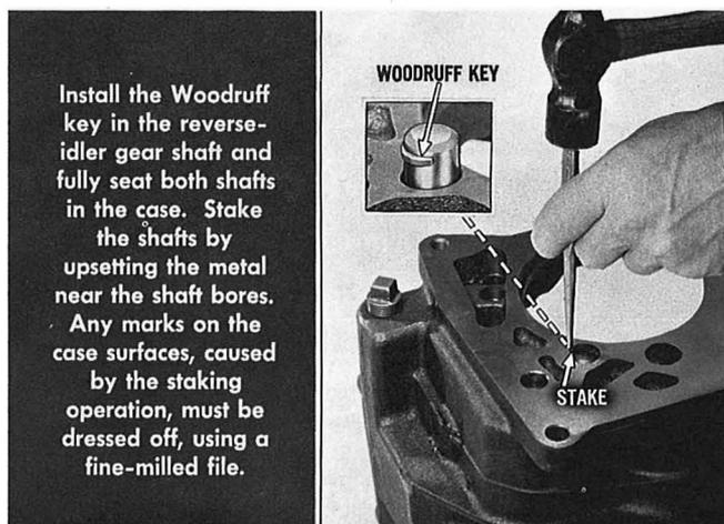
Install the Woodruff key in the reverse-idler gear shaft and fully seat both shafts in the case. Stake the shafts by upsetting the metal near the shaft bores. Any marks on the case surfaces, caused by the staking operation, must be dressed off, using a fine-milled file.
