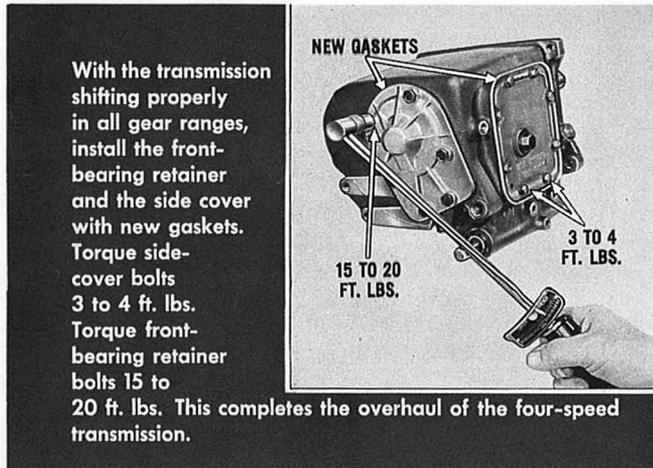
With the transmission shifting properly in all gear ranges, install the front-bearing retainer and the side cover with new gaskets. Torque side-cover bolts 3 to 4 ft. lbs. Torque front-bearing retainer bolts 15 to 20 ft. lbs. This completes the overhaul of the four-speed transmission.
