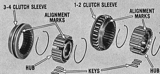
**Synchronizer Clutches:** Push the hubs out of the clutch synchronizer sleeves. The keys will fall clear. Remove the two tanged springs from each of the hubs. Note that the clutch sleeves and hubs are etched with alignment marks to insure correct assembly of matched units.
