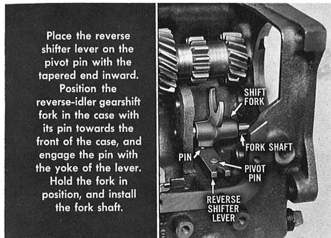
Place the reverse shifter lever on the pivot pin with the tapered end inward.
