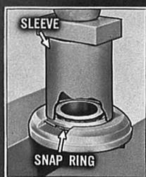
Caution should be observed to prevent damage to the bearing and retainer during removal and installation. A 2 3/4" O.D. sleeve will assist in removing the bearing and prevent damage to the new bearing during installation. This completes the inspection procedures.
