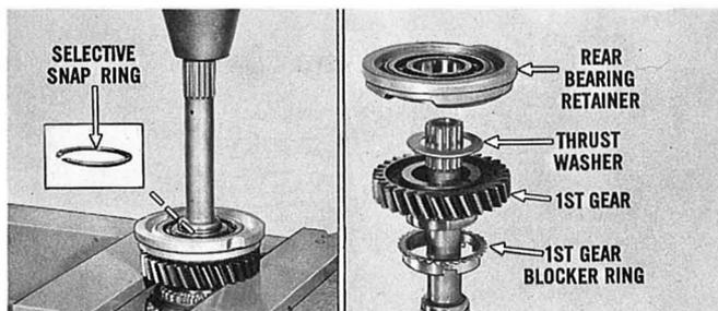
Remove the rear-bearing selective snap ring. Support the 1st-speed gear on suitable blocks, then slowly press the mainshaft out of the bearing bore. To avoid damage, the blocker ring must remain clear of the supports. Remove the 1st-speed gear thrust washer, the 1st-speed gear and the 1st-gear blocker ring.
