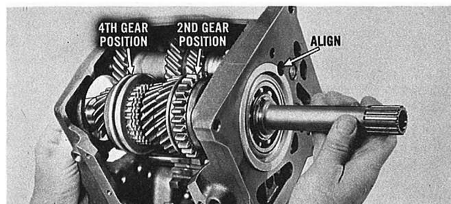
Shift the 3-4 synchronizer sleeve forward into 4th-gear position and the 1-2 synchronizer sleeve into 2nd-gear position. Then, insert the mainshaft through the case until the rear bearing retainer is flush with the rear face of the case. The clearance hole in the retainer and case must align.
