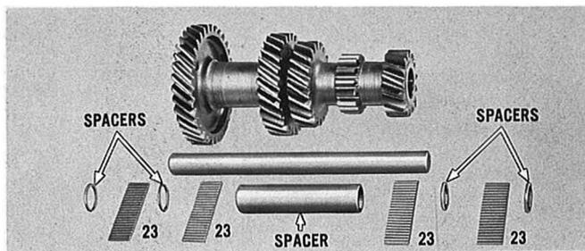
Remove the 92 needle bearings from the countergear (four sets of 23 each). All are  $\frac{7}{64}$ " in diameter and  $\frac{3}{4}$ " long. Inspect the bearings, spacers and the countergear shaft and bore for galling or excessive wear. Install new parts as necessary. Use petroleum jelly and the dummy shaft to assist in their installation.
