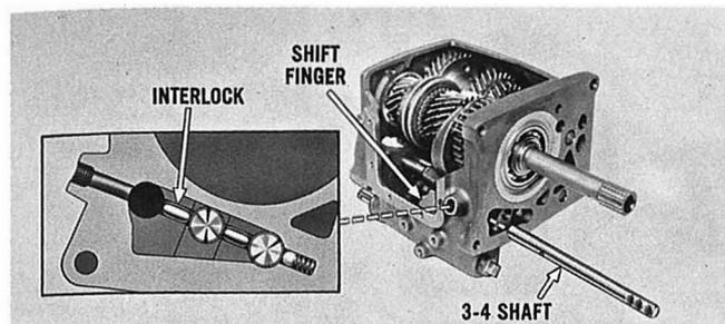
Drop the remaining interlock into the detent channel, and insert the 3-4 shift fork shaft partially into the case. The three detent notches should be up, facing away from the 1-2 shaft. If necessary, move the selector shaft so that the shift finger drops into the opening in the 1-2 shift fork gate.
