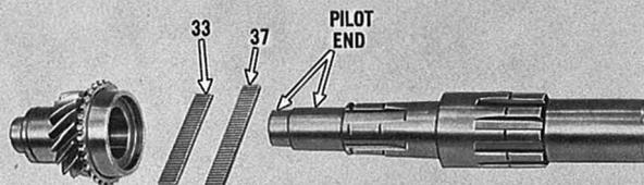
Remove the 37 outer needle bearings and the 33 inner needle bearings from the clutch gear bore. All are  $\frac{3}{32}$ " in diameter and  $\frac{1}{2}$ " long. Inspect the bearings, the clutch gear and the pilot end of the mainshaft for galling or excessive wear. Install new parts as necessary.
