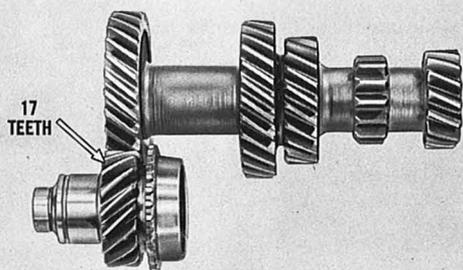
. . . Corvair 95 models (including the Greenbrier). If the clutch gear has 16 teeth, it must be replaced during assembly with part number 3785454, which has 17 teeth, in order for the countergear and clutch gear to mesh properly. All other mainshaft gears will mesh satisfactorily with the relieved countergear.
