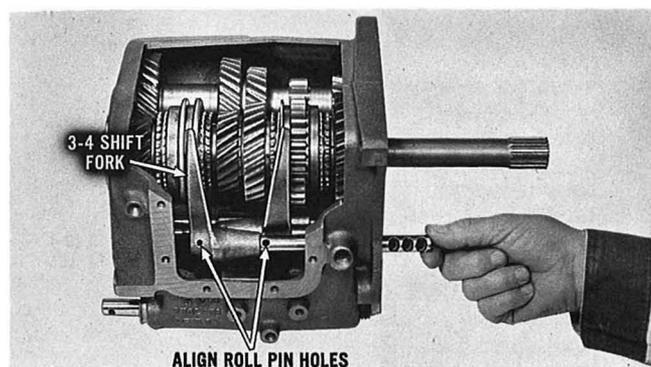
Engage the 3-4 shift fork with the synchronizer sleeve. Insert the shaft through the shift fork, and align the roll pin holes. Install the roll pin.
