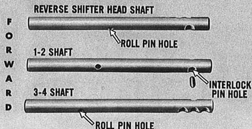
Before installing the 3 main shifter shafts, let's identify each. The reverse shifter head shaft has the roll pin hole almost centered on the shaft. The 1-2 shaft has an interlock pin hole drilled through the end of the shaft. The 3-4 shaft roll pin hole is nearest the forward end of the shaft.
