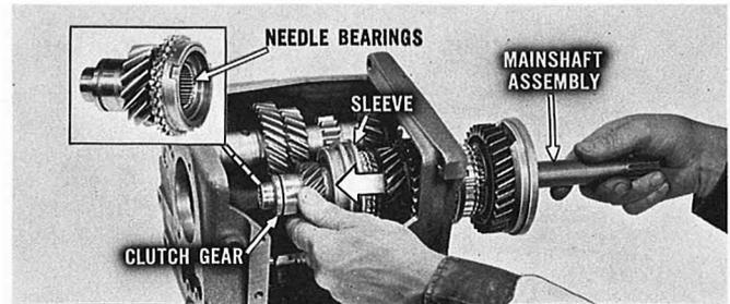
Shift the 3-4 synchronizer sleeve full forward (4th gear). Grasp the clutch gear and the rear of the mainshaft, and remove the complete mainshaft assembly from the case. **NOTE:** Be careful to prevent the clutch gear from separating from the mainshaft. There are 70 needle bearings inside the bore of the clutch gear.
