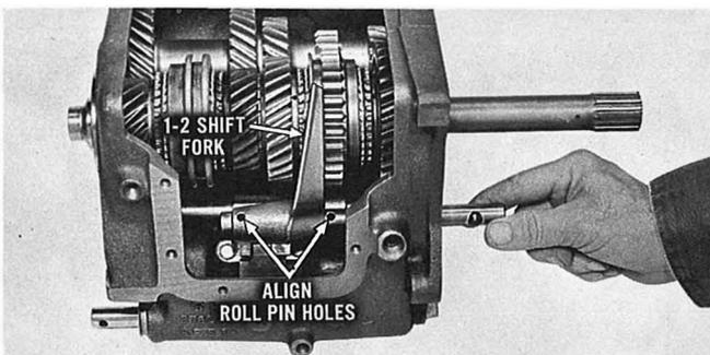
Engage the 1-2 shift fork with the 1-2 synchronizer sleeve. This shift fork is easily identified by the through gate. Push the shaft through the fork and align the roll pin holes. Install the roll pin.
