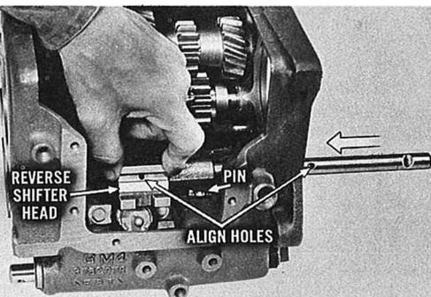
Engage the pin of the reverse shifter head with the yoke of the reverse shifter lever. Then, push the shaft into the case and through the bore of the shifter head until the roll pin holes align.
