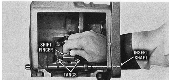
Coat the selector shaft and seal lips with petroleum jelly, and insert the shaft through the rear of the case. Attach the shift finger with cap screws. Bend the lock tangs against the heads of the cap screws. Install the drain plug.
