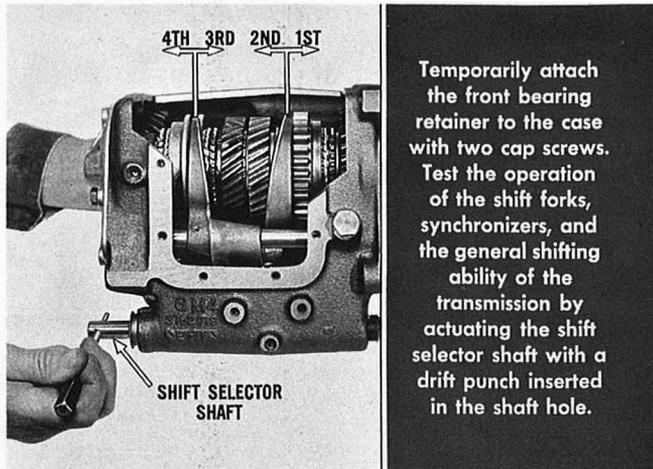
Temporarily attach the front bearing retainer to the case with two cap screws. Test the operation of the shift forks, synchronizers, and the general shifting ability of the transmission by actuating the shift selector shaft with a drift punch inserted in the shaft hole.
