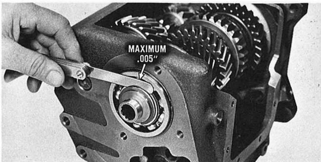
Measure the clearance between the bearing and selective snap ring. Maximum allowable clearance should be .005". This snap ring is available in three thicknesses, .084" — .087" and .093", to obtain correct clearance.
