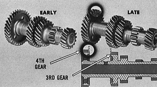
Inspect the inner faces of the 4th speed gear teeth and the 3rd-speed gear teeth on the countergear. If worn or badly galled, replace the early-type countergear with the late-type which has a .005" to .020" relief ground on the 4th and 3rd-speed gear teeth as shown.
