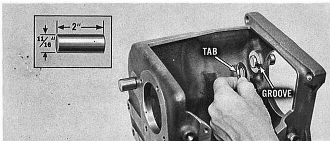
Coat both countergear thrust washers with petroleum jelly, and position each against the case with the tabs engaged in the case grooves. Two short pieces of rod ( $1\frac{1}{16}$ " O.D. x 2" long) inserted into the shaft bore, as shown, will help to hold the washers in position during countergear installation.
