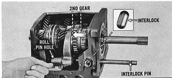
Shift the 1-2 synchronizer clutch sleeve full forward into 2nd gear. Drive the roll pin out of the 1-2 shift fork and shaft. Tap the shaft out of the case and remove the shift fork. Keep the interlock pin with the shaft. Remove the second of the two interlocks.
