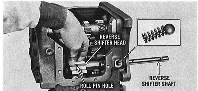
Drive the roll pin out of the reverse shifter shaft. Tap the shaft out of the case, and remove the shifter head. Remove the detent ball and spring from the bottom of the detent channel bore. **NOTE:** All detent springs and balls are identical.
