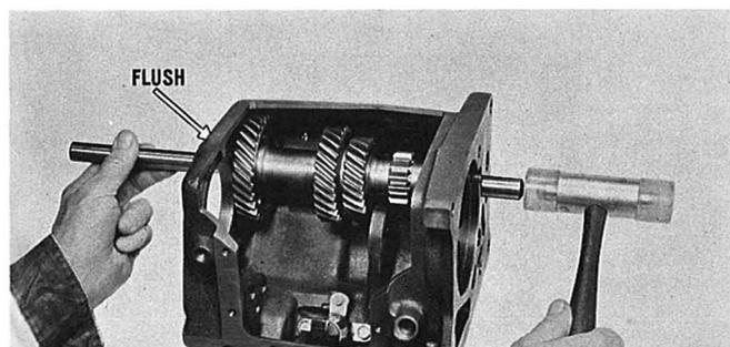
Push the countergear shaft into the rear of the case by hand. Then tap the countershaft with a soft-faced hammer until the shaft is flush with the front face of the case. The shaft is a slight press fit at the forward end. Turn the countergear by hand to check ease of rotation.
