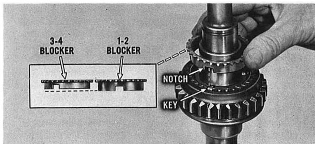
With the rearward end of the mainshaft held upright, position one of the 1-2 blocker rings in the synchronizer assembly. Engage the notches with the keys. **NOTE:** The 1-2 and the 3-4 blockers are slightly different. The 1-2 blockers have longer hubs.
