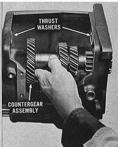
**Mainshaft:** Shift the synchronizer sleeves to their neutral position. Then, slowly lift the mainshaft straight upwards to prevent dislodging the clutch-gear needle roller bearings. Remove the spacer washer and the 4th gear blocker ring.
