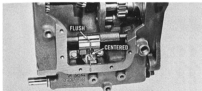
Install the roll pin until it is flush with the bottom face of the sliding gate. Move the shaft forward until it drops into the detent which centers the shifter gate opening with the inhibitor plunger. This will permit installation of the 1-2 shaft.
