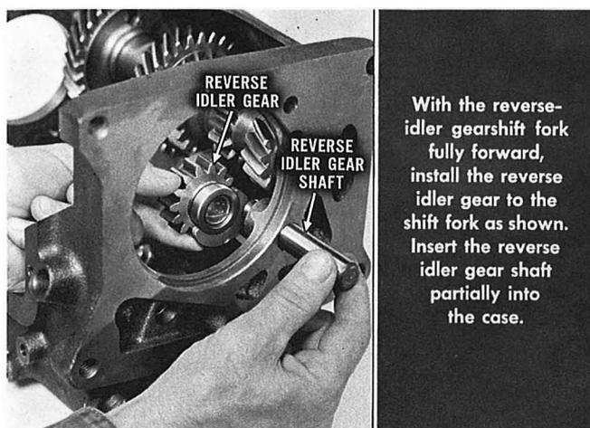
With the reverse-idler gearshift fork fully forward, install the reverse idler gear to the shift fork as shown. Insert the reverse idler gear shaft partially into the case.
