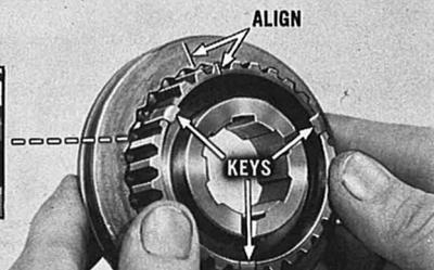
**Synchronizer Clutches:** Place two springs in each of the hubs so that the tanged end of each spring falls into the same keyway as shown. To assemble each unit, hold the three keys in position and align the etched marks. Slide the hub into the sleeve. The hook ends of each key must be located over the springs.
