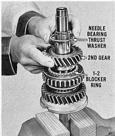
Clamp the mainshaft in the vise so that the forward end is up. Install the second of the 1-2 blocker rings, and engage the notches with the keys. Install the 2nd-speed gear with the clutching teeth downward. Place the needle-bearing thrust washer on the 2nd-speed gear.
