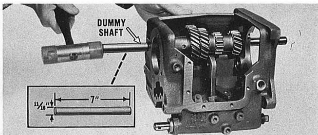
Using a drift punch, tap the countershaft a short distance out of the rear of the case. Then, using a locally made dummy shaft, tap the countershaft all the way out. The dummy shaft will keep the 92 needle bearings inside the countershaft bore from falling out of position as the countershaft is removed.
