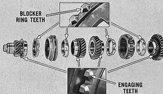
Inspect all blocker ring teeth and the engaging teeth of the synchronizer sleeves and matching gears. The teeth must be sharply defined and not rounded. Install new parts as necessary.
