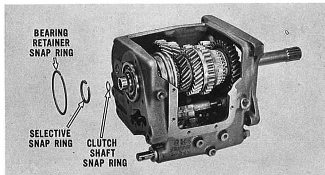
Remove the bearing retainer snap ring, the clutch bearing selective snap ring and the clutch shaft bottoming snap ring.
