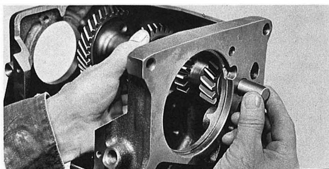
Insert the countergear assembly through the rear-bearing opening, and carefully lift the assembly into position between the thrust washers. Then, remove the two short pieces of rod.
