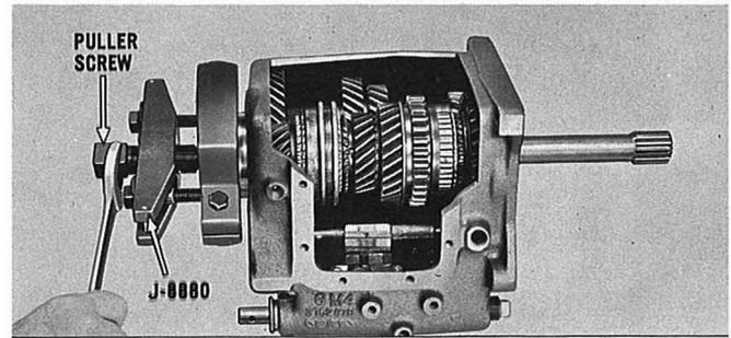
Install the clutch bearing puller plates, J-8880, into the bearing groove and the adapter plug into the clutch gear bore. Turn the puller screw slowly until the bearing is separated from the case. Remove the puller plates and adapter plug.
