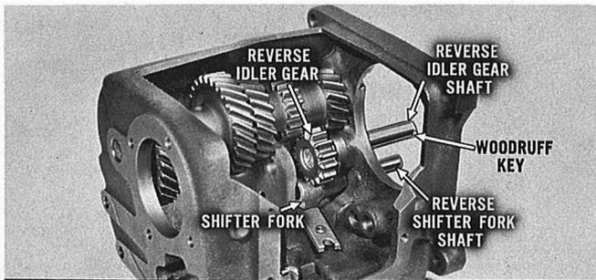
Remove both the reverse shifter fork shaft and the reverse idler gear shaft by tapping the shafts out of the case. The Woodruff key in the end of the reverse idler gear shaft prevents the shaft from rotating. Remove the reverse idler gear and the shifter fork.
