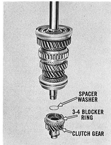
Place the clutch gear on the bench with the pilot bore upward. Place the second of the 3-4 blocker rings on the cone surface of the clutch gear, and locate the spacer washer over the needle roller bearings. Carefully insert the mainshaft into the clutch-gear bore. This completes the assembly of the mainshaft.
