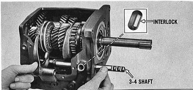
Tap the 3-4 shaft out of the case, and remove the 3-4 shift fork. Tip the case or use a magnet to remove the interlock from the detent channel. **NOTE:** The 3-4 shaft, 1-2 shaft and the reverse shaft can be removed from either end of the case.
