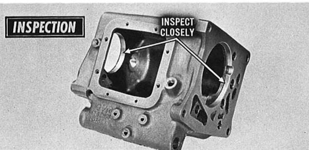
Wash the transmission case and all individual components in a good commercial cleaning solvent or clean kerosene. Air-dry, using compressed air. Inspect the case for cracks, especially near the front- and rear-bearing bores. Clean all old gasket material from surfaces of case and covers.
