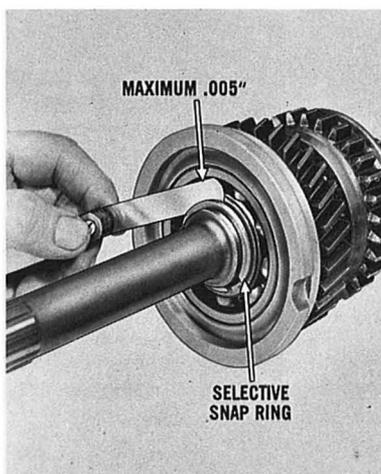
Install the selective snap ring. Measure the clearance between the rear face of the rear bearing and the snap ring. Maximum allowable end play should be .005". This snap ring is available in three thicknesses, .084" — .087" — .093", to obtain the correct clearance.
