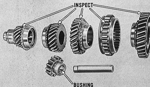
Inspect all gear teeth for chipping or excessive wear. Check the reverse-idler gear bushing as to shaft fit. Install new parts as necessary.
