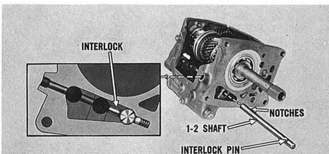
Shift the synchronizers to their neutral position, then install one of the interlocks in the 3-4 detent channel. Insert the interlock pin in the 1-2 shaft, and install the shaft partially into the case. The three detent notches at the forward end of the shaft must face towards the reverse shifter shaft.
