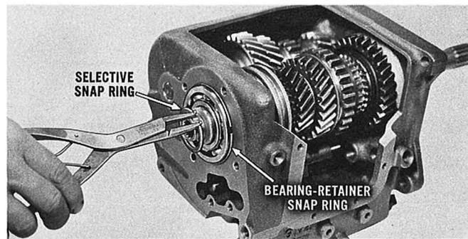
Install the front bearing (with snap ring) into the case, and tap around the outer edge of the bearing race until the snap ring seats against the case. Install the selective snap ring in the clutch gear groove.
