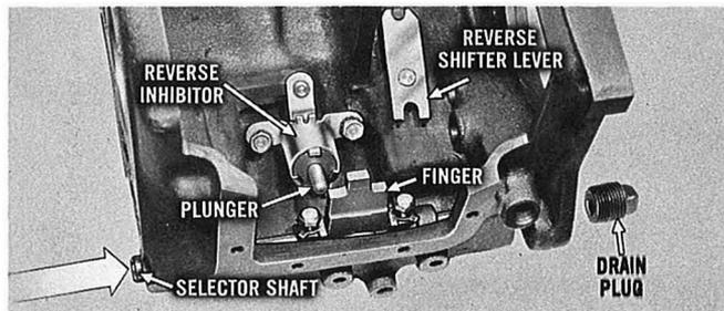
Remove the reverse shifter lever from the pivot pin and the drain plug. Remove the selector shaft finger and tap the selector shaft out of the rear of the case. Remove the reverse inhibitor with its plunger by removing the cap screws. This completes the disassembly of the case. The reverse inhibitor on . . .
