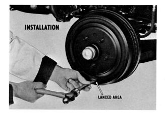
If linings and drums are severely worn, the shoes must be retracted to permit drum removal. On 1963 models, a lanced area on the face of the drum must be knocked out to gain access to the star wheel. Replace with a snap-in-type hole cover.
