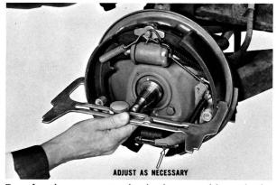
Transfer the gauge to the brake assembly with the opposite side of the gauge fitted over the shoes. Hold the actuating lever away from the star wheel, and turn the star wheel as necessary until the linings just touch the gauge.
