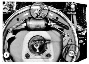
When there is only a slight clearance between the linings and the drum, such as when the brakes are correctly adjusted, the shoes rotate only a slight amount and the actuating lever does not move far enough to advance the star wheel. Therefore, the brakes cannot become overadjusted and lock up. Now, let's see how the override pivot plate functions.
