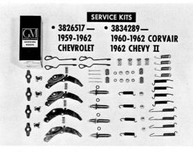
The self-adjusting mechanism is now available in two service kits, for converting the earlier Chevrolet, Corvair and Chevy II models from standard to selfadjusting brakes. New brake shoes are not included in these kits. Now let's follow the procedures to install a conversion kit on the 1961 Chevrolet.
