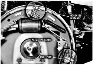
This increases the distance from the anchor pin to the actuating lever pivot point. Since the wire link maintains a fixed length, it, in effect, pulls the actuating lever to the position shown.
