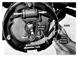
Position the actuating lever assembly to the secondary shoe. Place the return spring over the tang. Install the hold-down spring sleeve, spring and the deep dished washer, using a new longer pin. These new parts are included in both conversion kits.
