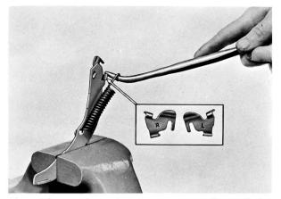
Clamp the actuating lever in a vise and install the pivot plate and override spring. The pivot plates are clearly identified for the right and left sides of the car. During a brake reline on the 1963 models, it is not necessary to disassemble the actuating lever assembly unless parts are damaged.
