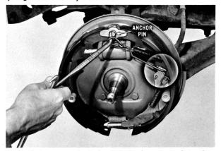
Hook the open end of the link in the pivot plate slot. Snap the link into position over the anchor pin.
