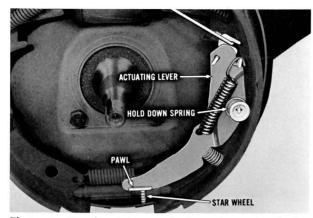
The actuating lever is attached to the web of the secondary shoe by the hold-down spring and pin, which also holds the pawl in firm contact with the adjusting screw star wheel. Now, let's see how this mechanism operates, using the left front brake.
