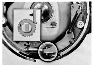
. . . moves outboard as it follows the curve of the star wheel. When the brakes are released, the pawl slips back over the teeth and takes a new bite on another notch.
