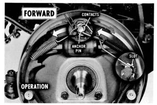
During a forward stop, the shoes rotate with the drum until the web of the secondary shoe contacts the anchor pin. Since the actuating lever moves forward with the secondary shoe, the open end of the wire link slides in the pivot plate slot. As a result, brake adjustment remains unchanged.
