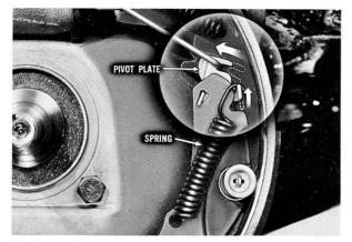
If the adjusting screw threads should ever bind or lock, preventing movement of the actuating lever, only the pivot plate rotates forward against spring tension.
