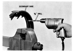
Remove the shoe assembly. When there is still usable lining material, the secondary shoes can be modified for attachment of the self-adjusting mechanism by drilling out the hold-down pin hole to  $\frac{3}{8}$  inch. If *new* brake linings are required, use the appropriate 1963 brake shoes.
