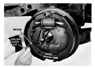
Install the primary brake shoe hold-down pin, the spring washer, the spring and shallow dished cup. A new spring washer, spring and cup are included in both conversion kits.
