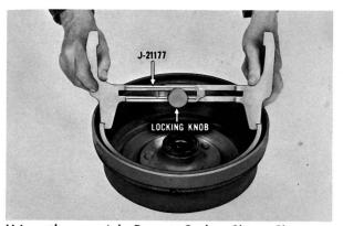
Using the special Drum-to-Brake – Shoe Clearance Gauge, J-21177, measure the brake drum diameter across the drum center line. Tighten the locking knob to hold this measurement.
