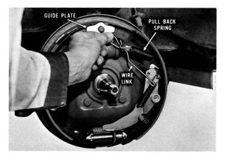
Install the brake shoe guide plate. This part is not used on the Corvair or Chevy II models. Install the secondary shoe pull-back spring, and connect the spring to the heavy wire link.
