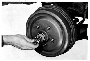
Install drums and all wheels. Check fluid level in the master cylinder and add if necessary. Road-test the car. Firmly apply the brakes several times in forward and reverse stops. This completes the installation procedures.
