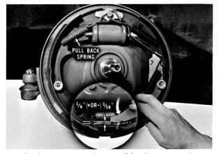
Install the primary shoe pull-back spring. Proper assembly is indicated when the bottom edge of the lever is  $\frac{1}{4}$  inch, plus or minus  $\frac{1}{4}$  inch above the center line of the adjusting screw. Check the actuating lever assembly by hand operation.
