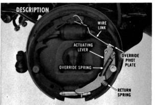
The self-adjusting mechanism consists of a heavy wire link, a pivoted actuating lever, an override pivot plate, an override spring, and a return spring.
