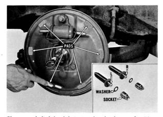
Clean and lightly lubricate the brake pads. New adjusting screw assemblies are included in the conversion kits, but on 1963 models the original adjusting screws must be cleaned and lubricated. Assemble with the antifriction washer and the socket. Left and right sides are identified by the *L* or *R* stamped on the adjusting screw.
