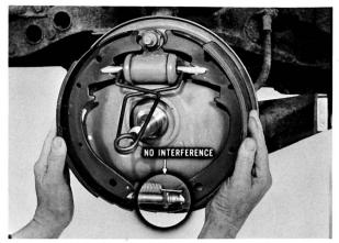
Connect the brake shoes, the adjusting screw and the adjusting screw spring together, and position this assembly to the anchor pin. The adjusting screw is correctly installed when the star wheel is nearest the secondary shoe. The spring is correctly installed when the coils do not interfere with the star wheel.
