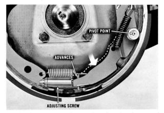
As the lever pivots, the pawl end rocks down and advances the star wheel, increasing the length of the adjusting screw. When the pawl turns the star wheel, it also . . .
