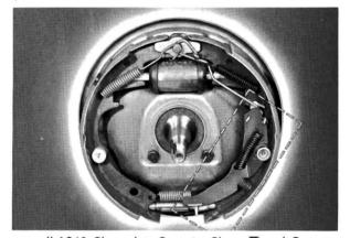
... all 1963 Chevrolet, Corvair, Chevy II and Corvette models incorporate another kind of brake improvement, new automatic, self-adjusting brakes. This new feature maintains a nearly constant lining-to-drum clearance throughout the life of the linings. Now, let's examine the parts which make up this assembly.
