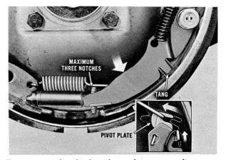
To protect the brake shoes from overadjustment, the star wheel can only advance a maximum of three notches during one stop, before the tang butts against the secondary shoe. Any additional shoe motion is absorbed by rotation of the pivot plate. This completes an explanation of how the self-adjusting mechanism operates.
