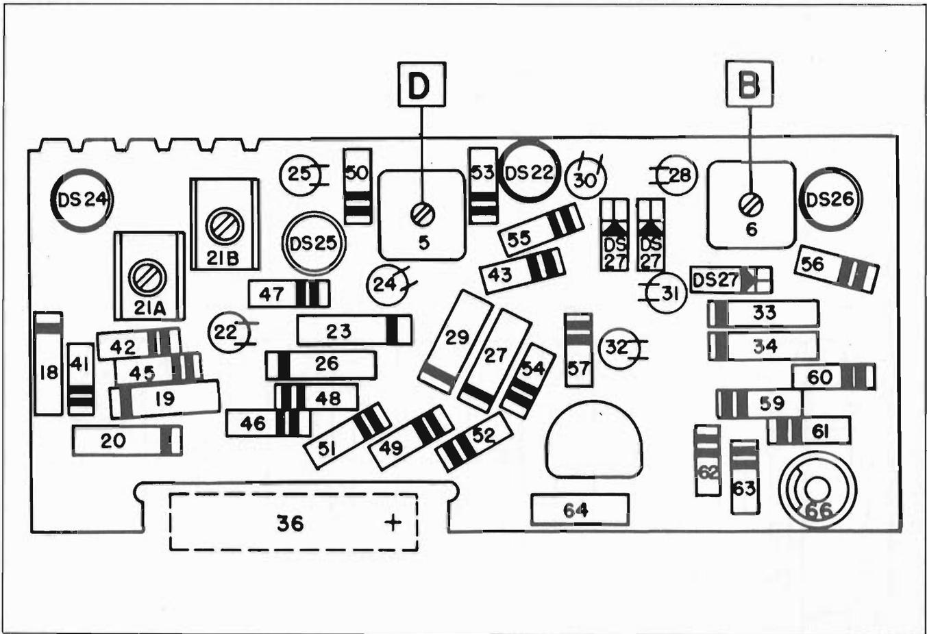
Figure 73 PARTS LAYOUT ON CIRCUIT BOARD - 985443 - RADIO
