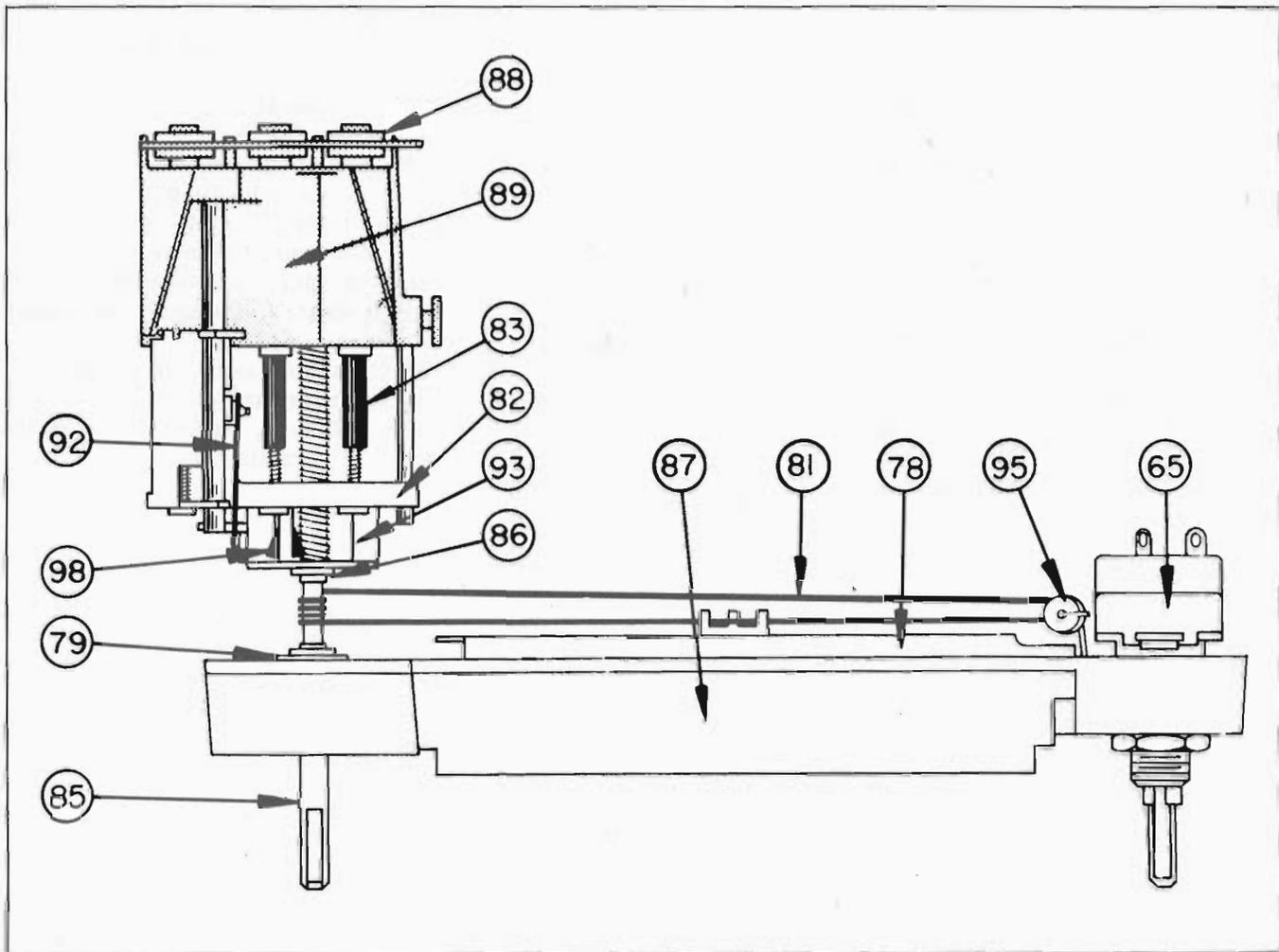
Figure 74 TUNER AND DIAL CORD VIEW - 985443 - RADIO
