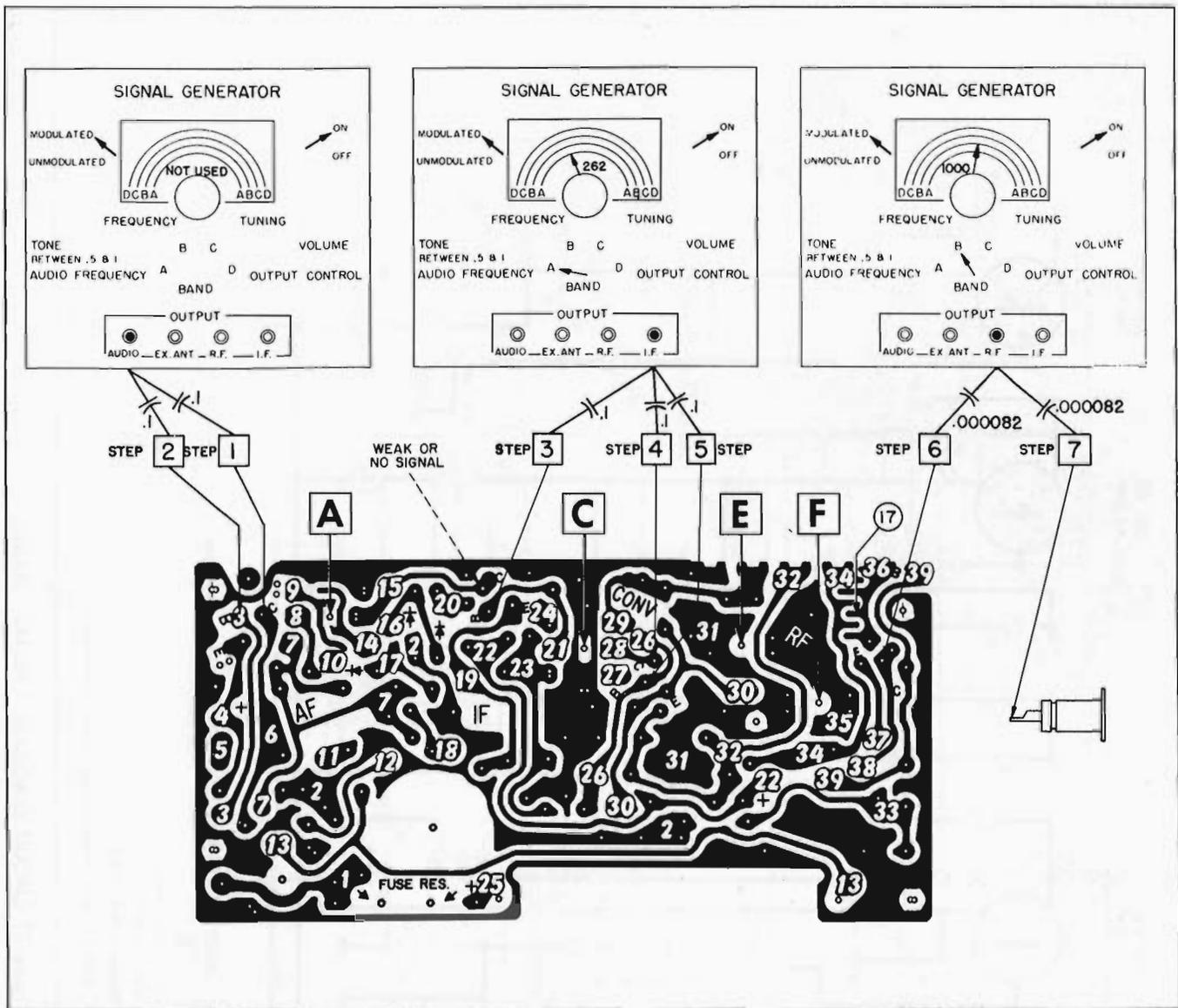
Figure 70 ISLAND NUMBER AND SIGNAL TRACING OF CIRCUIT BOARD - 985443 RADIO
