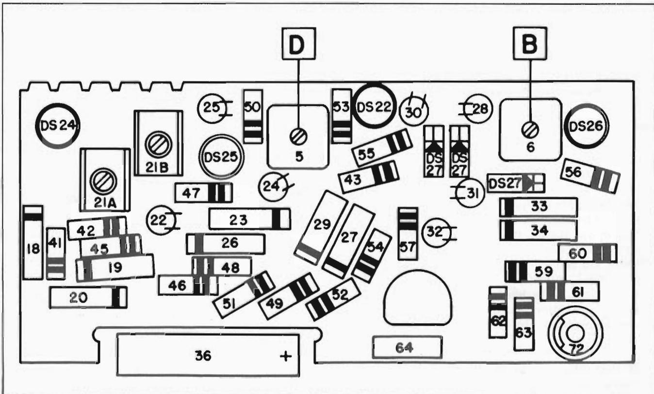
Figure 10 PARTS LAYOUT ON CIRCUIT BOARD - 985432 - RADIO
