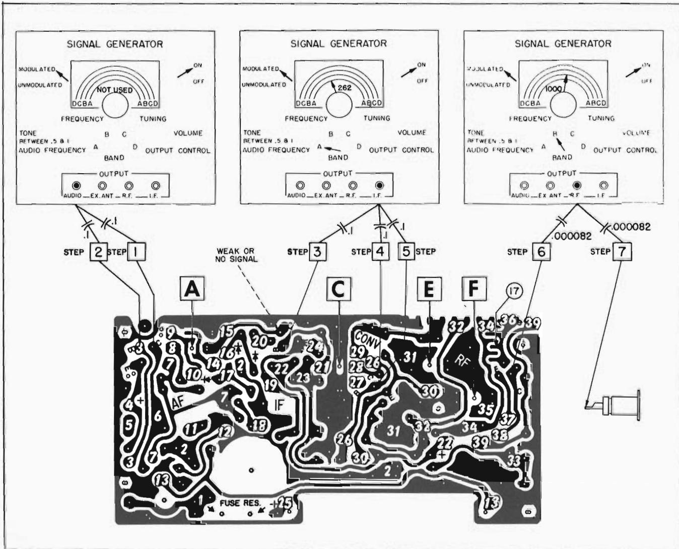
Figure 7 SIGNAL TRACING LOCATIONS ON CIRCUIT BOARD - ALL PUSH BUTTON AND MANUAL RADIOS
