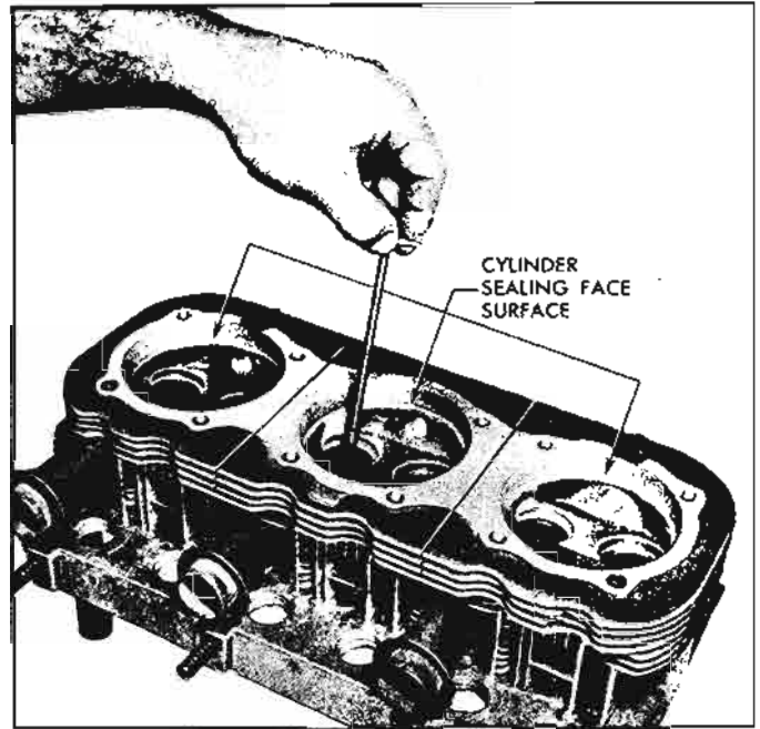
Fig. 6A-55—Cleaning Valve Bores, Using Tool J-8101
