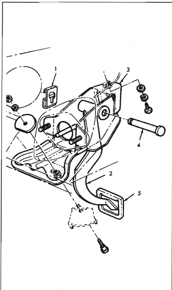
Fig. 5-7—Brake Pedal and Attaching Parts
