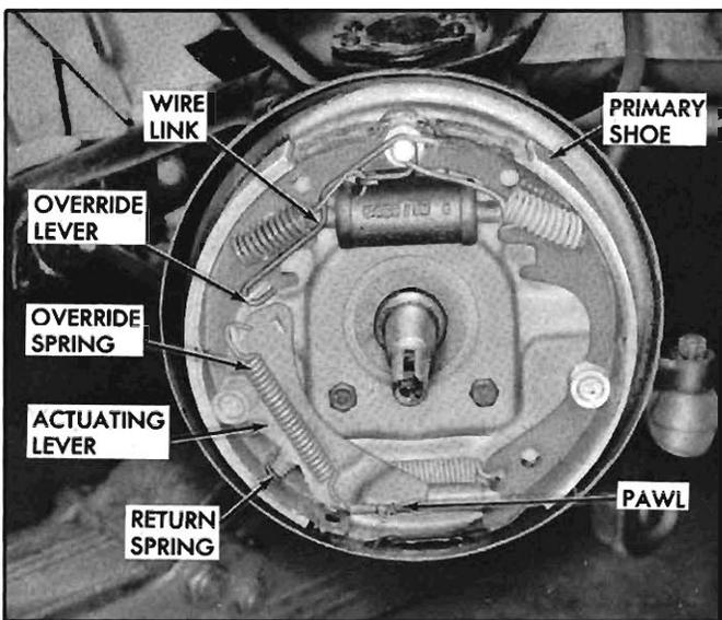
Fig. 5-1—Self-Adjusting Brakes
