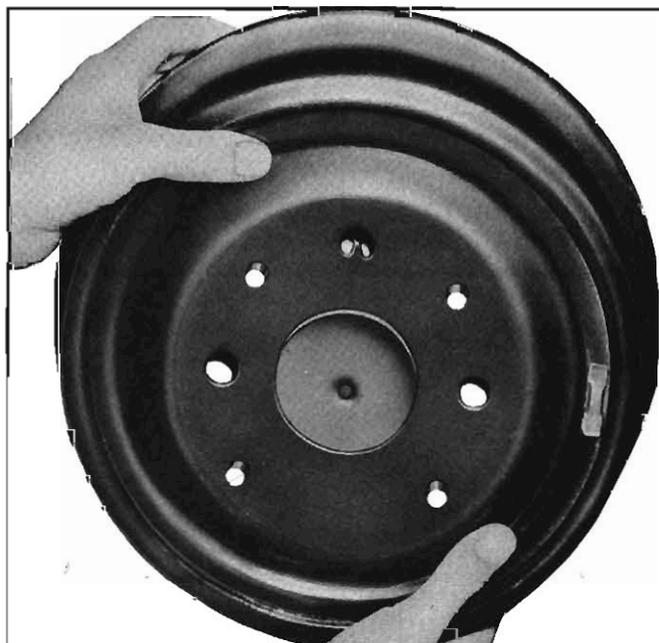
Fig. 5-14—Aligning Drum Tang with Axle Shaft
