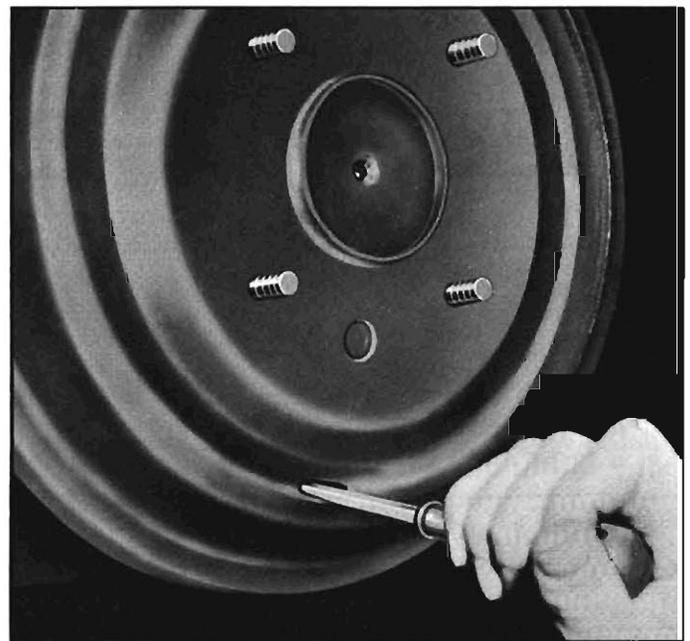
Fig. 5-2—Brake Drum Access Hole
