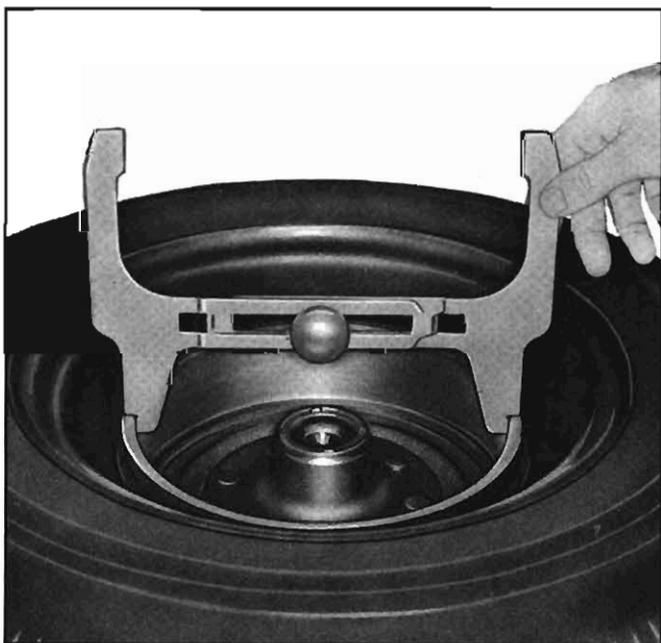
Fig. 5-12—Using Drum-to-Brake Shoe Clearance Gauge
