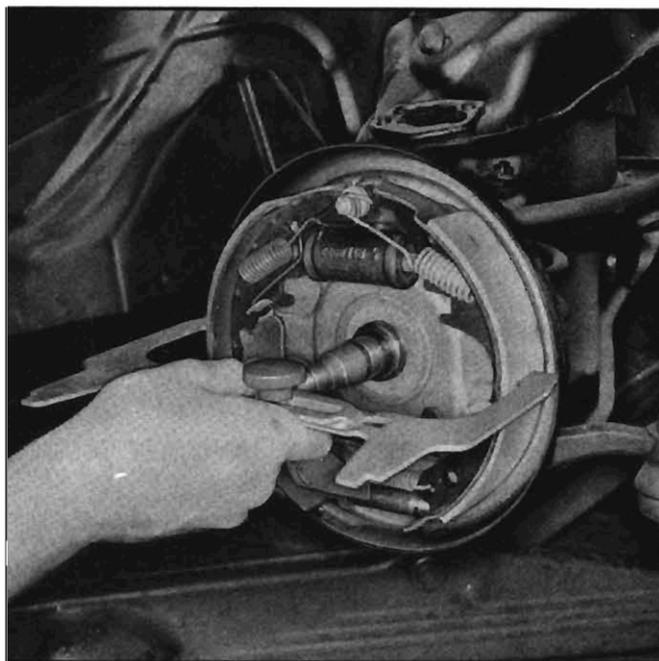
Fig. 5-13—Checking Brake Shoe Lining Clearance
