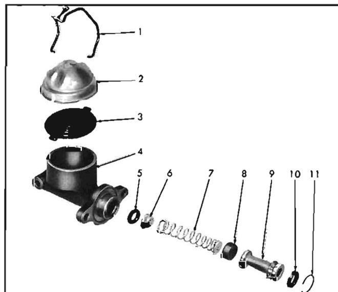
Fig. 5-6—Brake Main Cylinder
