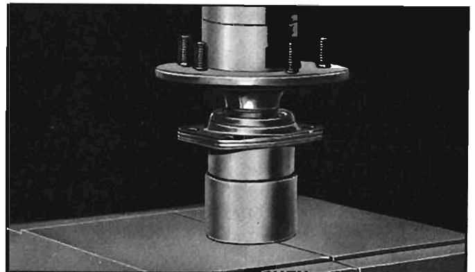
Fig. 6C-7—Installing Bearing Shield
