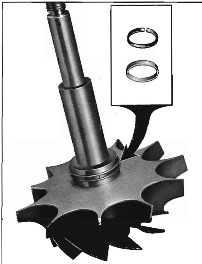
Fig. 52—Compressing Ring, Using Plastic Installer Ring
