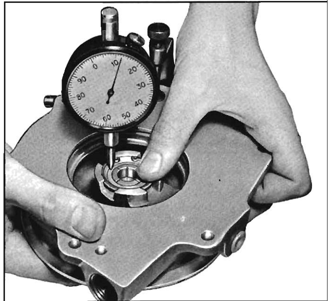
Fig. 48—Gauging Bearing-to-Housing End Play
