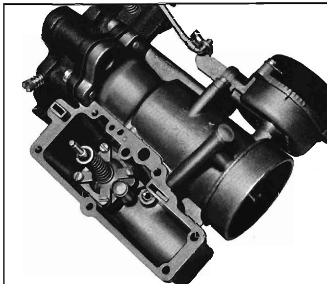
Fig. 35—Pump Diaphragm and Metering Jet Installation
