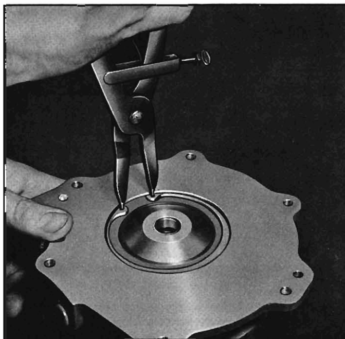
Fig. 44—Oil Seal Retainer Ring Removal
