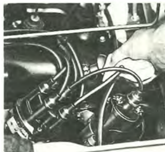
Checking for Spark
