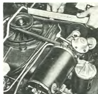
Checking Fan Belt Tension
