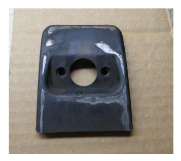
This is the backing plate that provides reinforcement as well as "nuts" for the door handle base.
