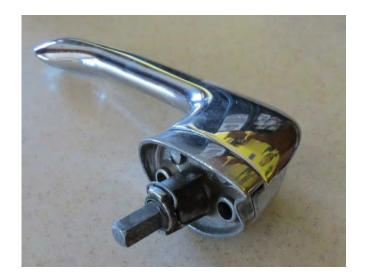
This shot is just to give a view of the handle out of the door to show how the handle is held on.
