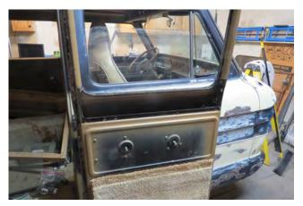
The small panel below the window must be removed. Although I already had the widow out, I am fairly certain that it does not have to be removed - just roll it up.
