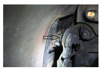
The first thing is to remove the clip that holds the handle on. It's just a simple widow/door handle clip used on so many GM cars of the era. Not the easiest to get to, but it becomes a little easier if a piece of wire is fashioned into a small hook to pull it out.
