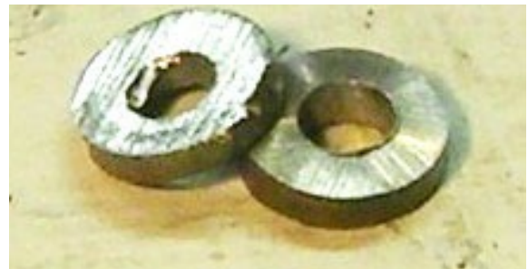
Two hardened steel doughnuts cut from the rocker arm stud.
