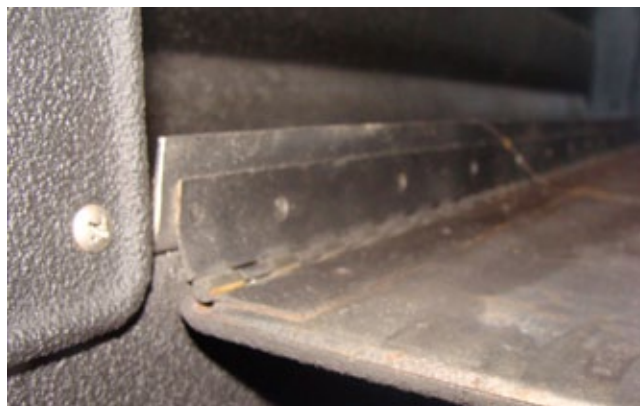
Here is a picture of the hinge joint all finished and showing how it has bent a little to allow for the extra thickness of the Line-X.
