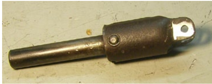
The Coupling separated from the end of the shaft.
