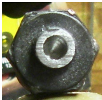
Rocker arm stud center drilled with #2 bit
