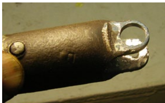
Drill out the holes in the coupling to fit the bushings (doughnuts) that you are going to make.
