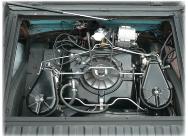
New wires, new lines, new paint and a hinged lid.
