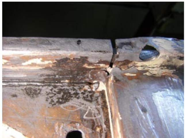
I plan to expose all four clip areas and then Acid etch the rusty stuff; followed by Epoxy and the final paint. I am toying with the idea of a black Rampside with a Silver stripe, roof and wheels.
