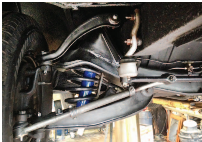
Left: New springs and shocks are installed.
