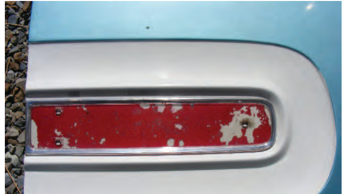
Deteriorated original-type reflector
