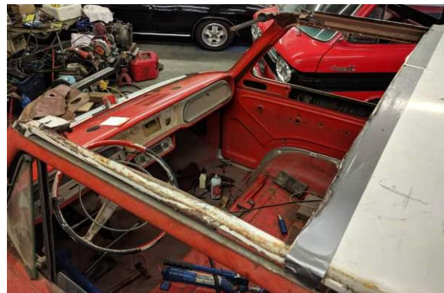
Drivers side top view of damaged roof skin and bracing cuts.
