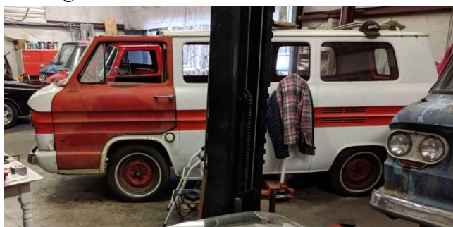
Side view with undamaged drivers door fitted for alignment.
