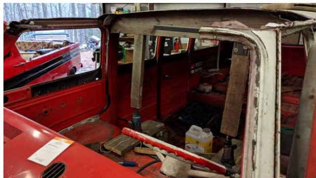
Drivers side front with alignment braces temporarily installed.
