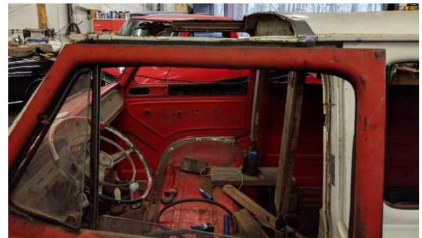
Alignment reference top of door and roof is almost there.
