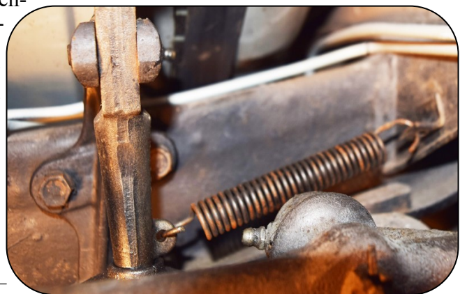
Figure 5. Early design shifter stabilizing spring.
