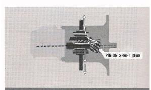
The pinion shaft gear drives the ring gear on the differential case in the conventional manner, delivering power to the rear axle shafts and in turn to the rear wheels.
