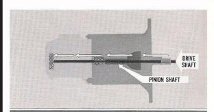
Engine power is delivered to the transmission by a drive shaft which passes through the hollow pinion shaft of the differential, and enters the rear of the transmission case. This shaft continues through to the front of the transmission.
