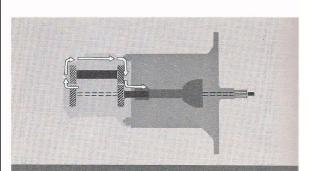
Power returns through the transmission the same as in a normal 3-speed unit. (Second speed gear is illustrated.) The output shaft resembles a sleeve over the input shaft, and is splined into the hollow differential pinion shaft.
