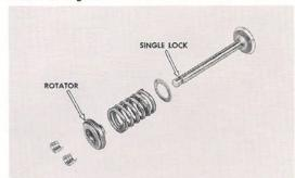
Corvair 95 engines for 1963 and '64 are equipped with single lock design stellite exhaust valves and rotators which are now available for installation in earlier Corvair 95 vehicles. Now let's look at recommended grinding angles.
