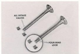
All intake valves have the single groove lock. However, when the original exhaust valves need replacement, you should use the four bead lock design on all except the Corvair 95 engines.
