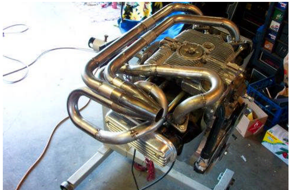
Air-cooled horizontally-opposed 4-cylinder Volkswagen 412 engine with mandrel-bent pipes and 4-into-1 merge collector.
