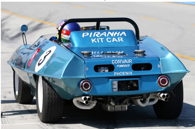
Corvair-powered Piranha owned by Dick Carbajal. This is one of the cars built by AMT. Note the 1965 Corvair tail-light lenses, headers, and deep-sump oil pan.
