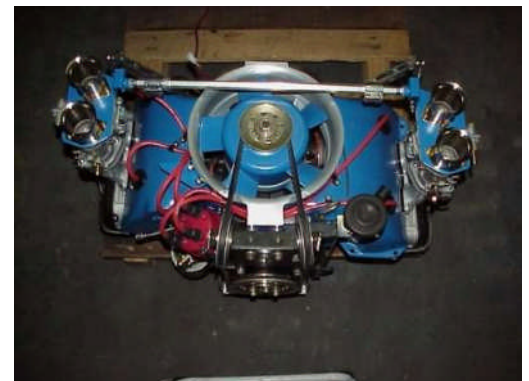
Another variation of a horizontal fan kit, this one offered by Reichert of Germany.
