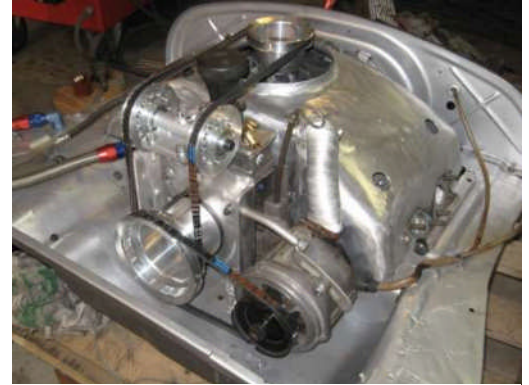
CFR Tangerine Racing Horizontal Cooling Fan Kit installed on a Porsche 914 / Type 4 engine.
