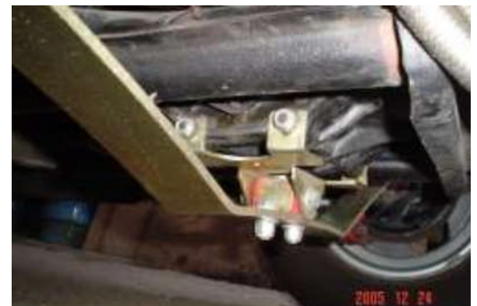
Camber compensator on a dune buggy. Spring pivot is bolted to the differential.
