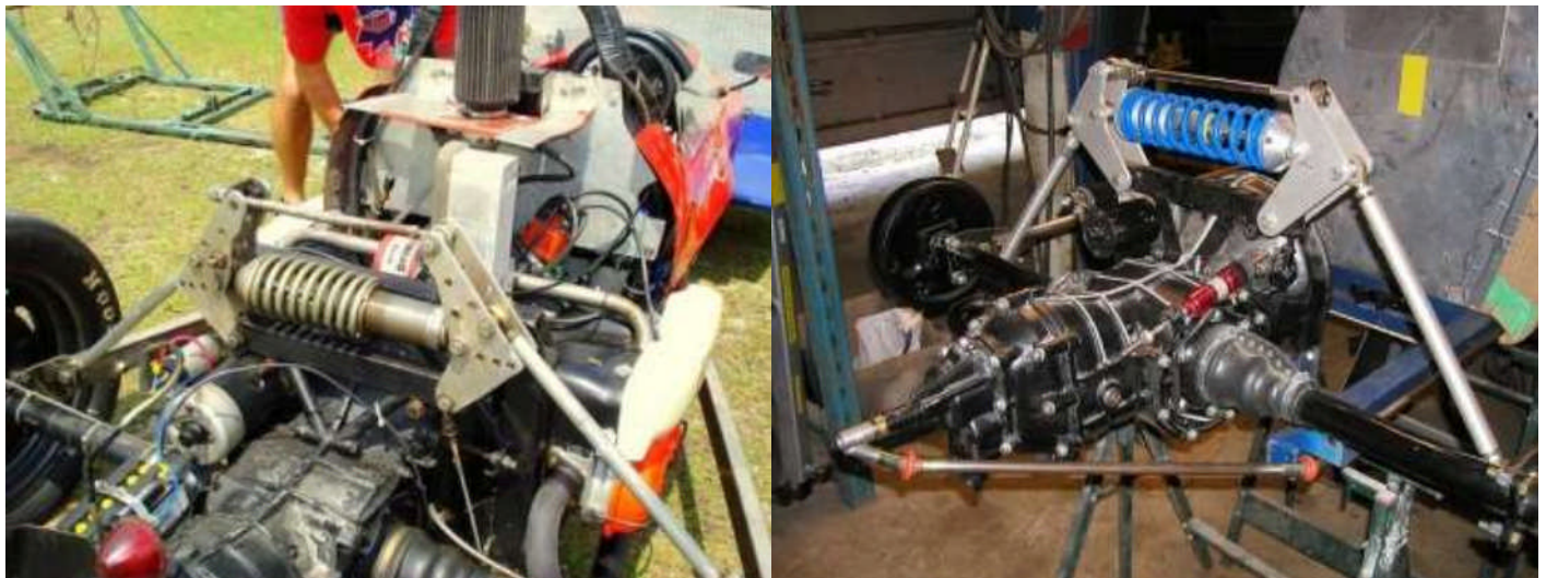
Two photos of zero-roll resistance swing axle suspensions on Formula V cars. The wheels are suspended against each other instead of to the chassis.
