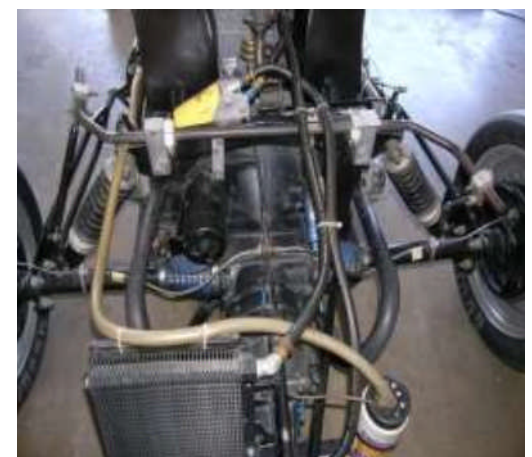
Z-bar on an older Formula V car. The bar pivots in the clamps bolted to the chassis.
