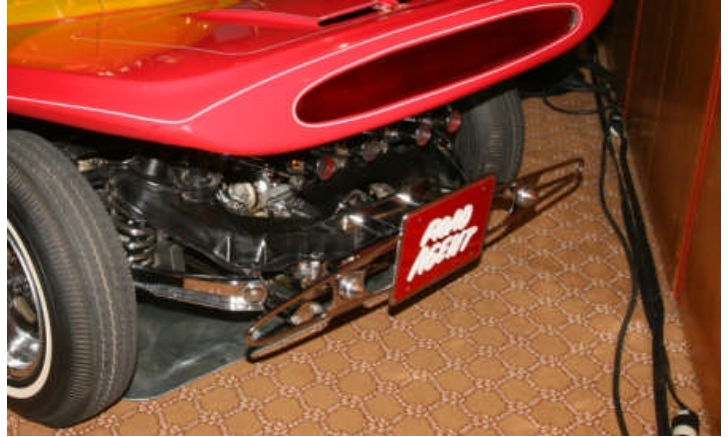
That's right. The entire power-train is reversed, front-to-rear, so that the Corvair suspension trailing arms become leading arms instead!
