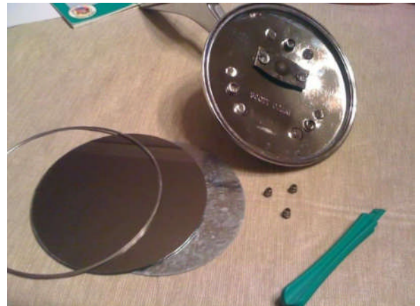
In some cases, the mirror glass is secured to the mirror head with a spring ring.
