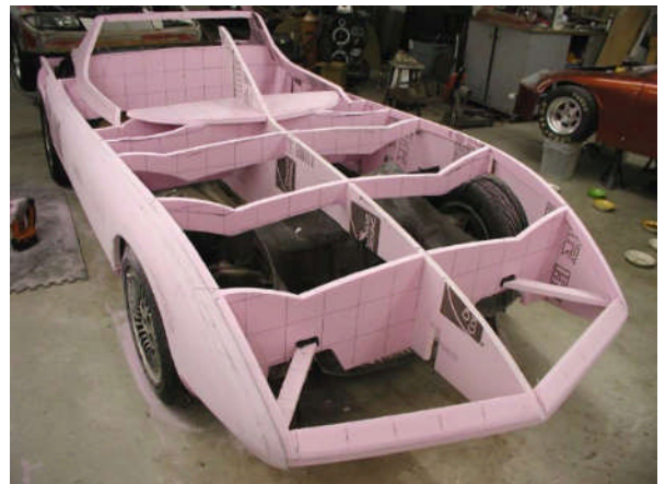
Building up the body buck with foam panels.
