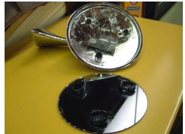
In other cases, the glass is simply glued-on. Photo by Mike Tarrant of Prescott, AZ.
