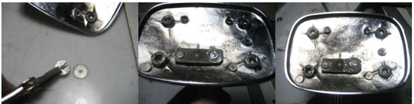
Glenn Davis of Peekskill, NY repaired his Corvette mirrors by inserting a slotted steel washer under the peened head of the stud that secures the spring plate. Then, for extra measure, he swabbed it with JB Weld for a permanent fix.
