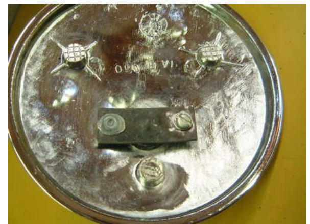
Here is the little spring plate that puts the ball-and-socket in compression. On the left side, the factory peened the top of the stud over the plate, just like the head of a rivet. On the right side, the plate is held down with a screw. This is one of the three kinds of repairs described in our article.
