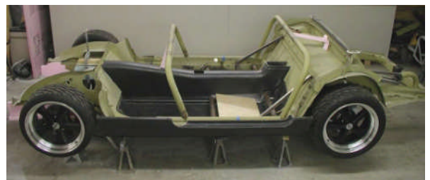
The rolling platform prior to body fabrication.
