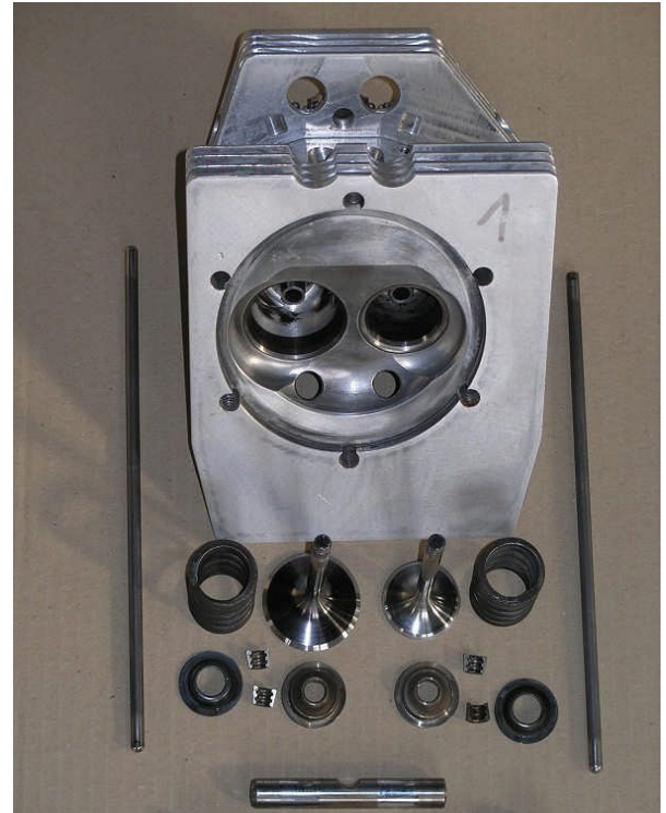
Individual cylinder head for each cylinder barrel. Dual spark plugs for each cylinder. Huge cooling fins. Push rods with rockers.
