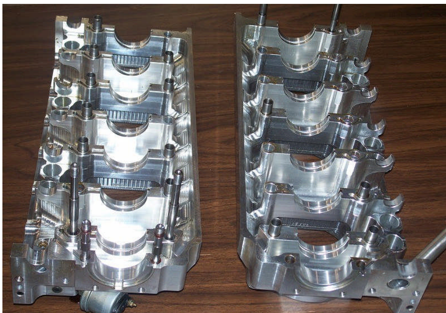
The Jubira 3300. The entire crankcase is CNC-machined aluminum! 7-main bearings. Camshaft rides in the crankcase like a Corvair.
