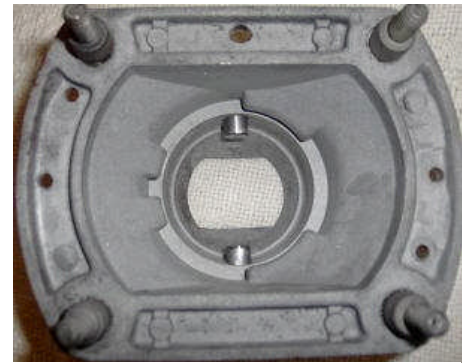
Disassembled shifter base (29). The two pins in the center may be worn.
