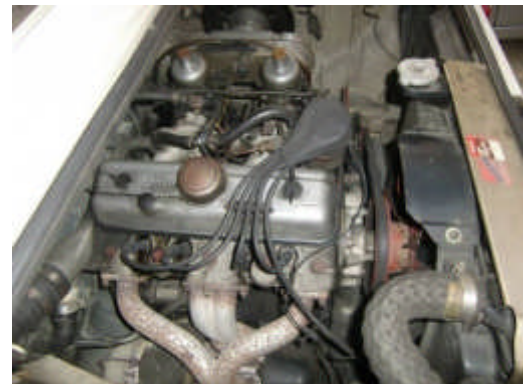
Dual carb slant-four water-cooled engine.
