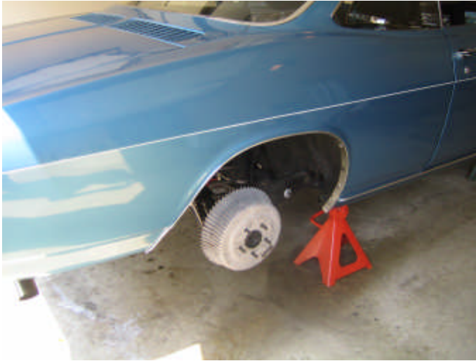
Wheel studs in. Brake drums on. The studs should align perfectly with the holes in the drums.
