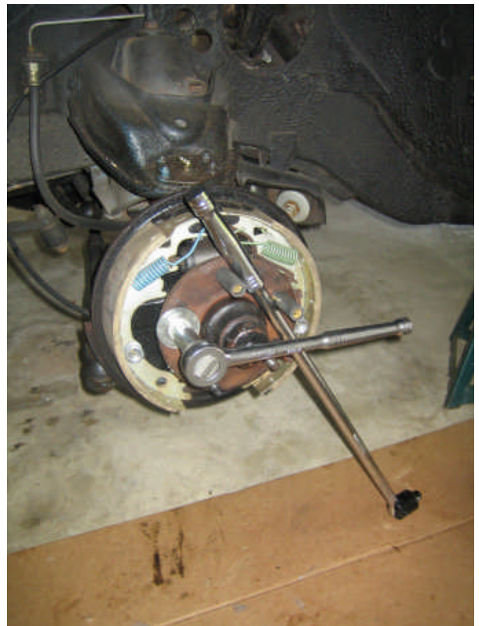
Pulling-in a new wheel stud. The long breaker bar touching the floor prevents the hub from turning.
