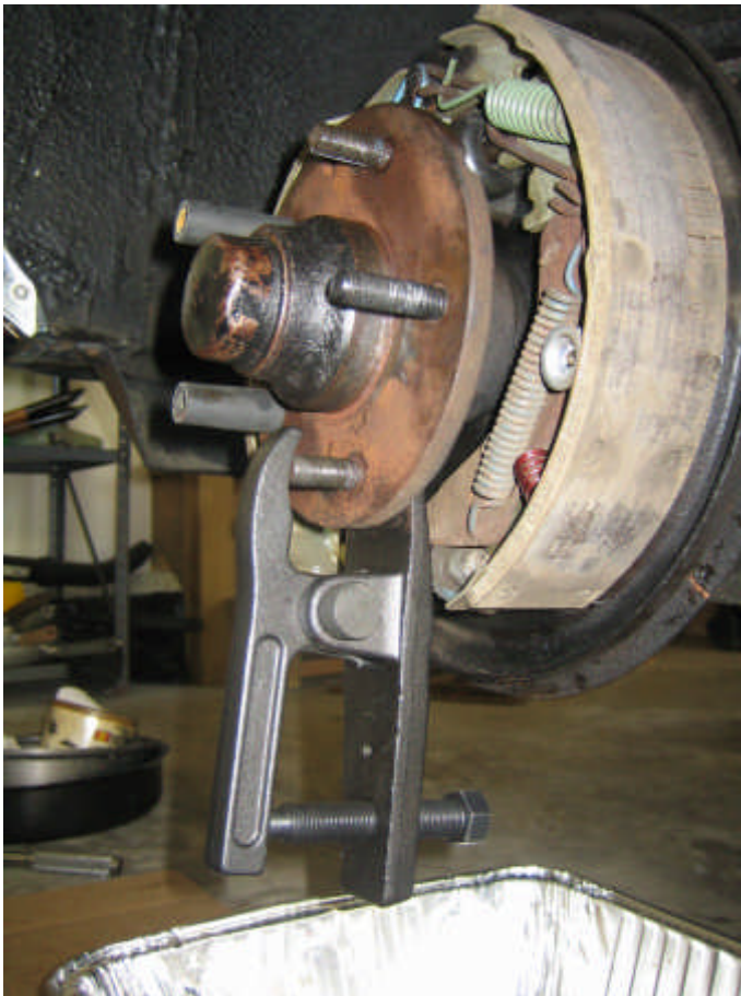
Popping out the old wheel studs with the Harbor Freight "Forged Ball Joint Separator".
