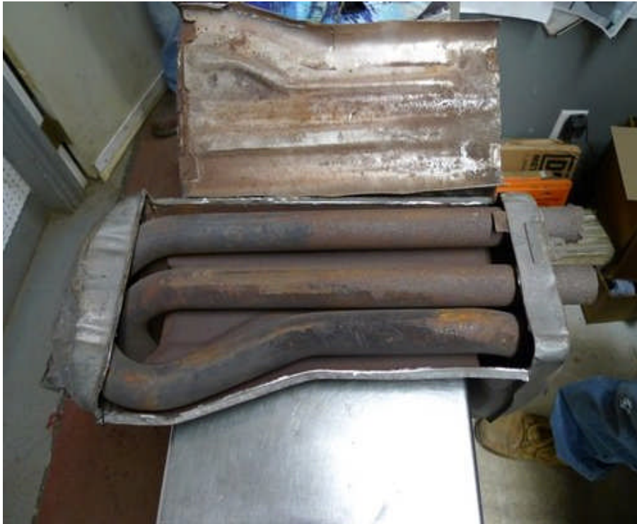
Like Volkswagen, Porsche equipped its 356 coupes and cabriolets with heat exchangers starting in 1963, but only for the German and Swedish markets. American buyers continued to get the "Stale Air" setup until the 911 arrived in 1965. The photo above shows the Porsche 356 heat exchangers, which are much larger (and therefore much more effective) than the Volkswagen equivalents.
