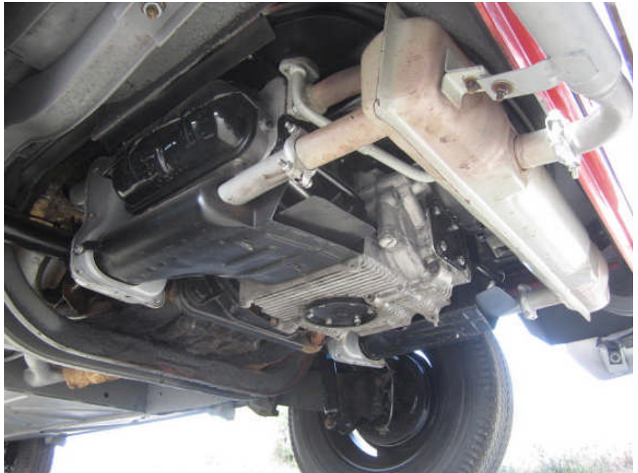
Early Volkswagen "Stale Air" heating system took cooling air from the bottom shrouds of the engine and pumped it directly into the passenger cabin of the car. Note the thermostatically-controlled flaps at the rear of the shrouds. Chevrolet engineers copied this design for the Corvair "Direct Air" heating system.
