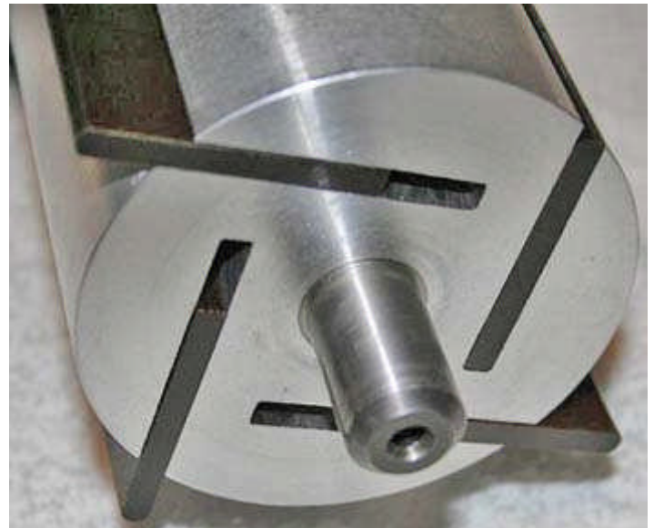
Judson supercharger rotor showing the sliding vanes. Lubricated with Marvel Mystery Oil!
