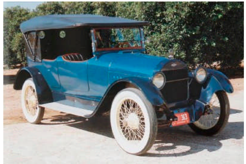
The original Chevy V8. 1917 Chevrolet D Series. 288 cubic inches. 55 horsepower.
