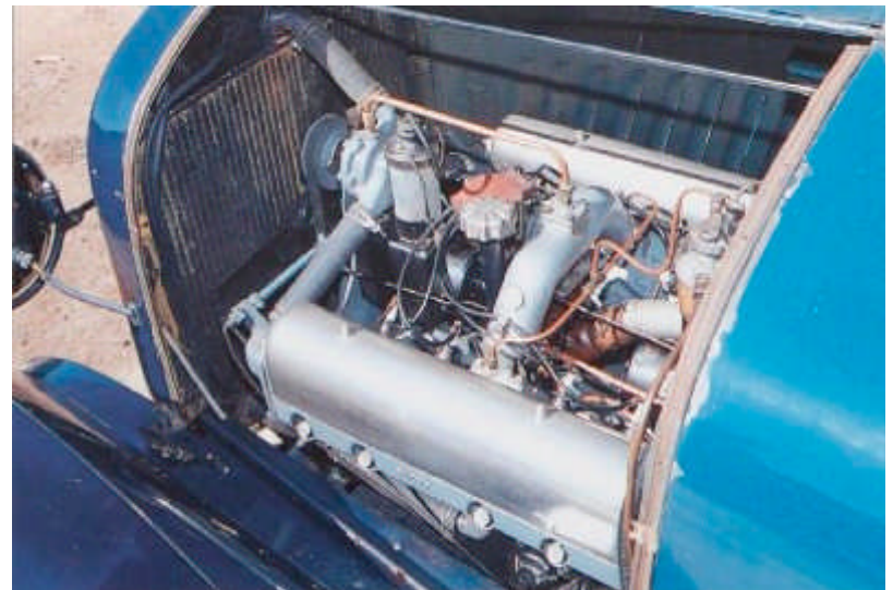
The original Chevy V8. 1917 Chevrolet D Series. 288 cubic inches. 55 horsepower.
