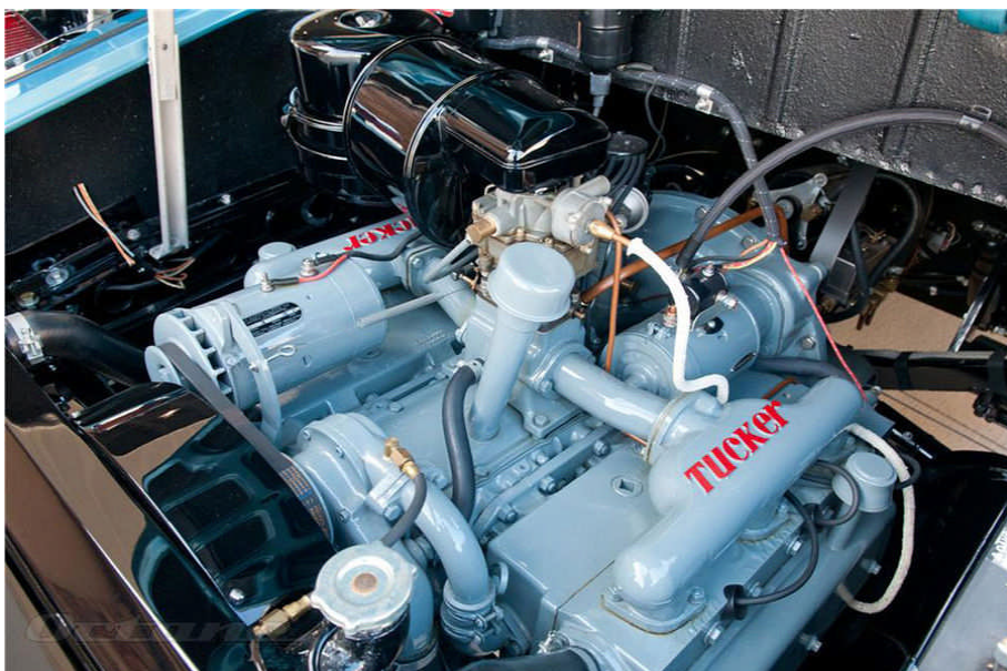
Below: Water-cooled version of the Franklin OC-335 as equipped in the Tucker automobile.
