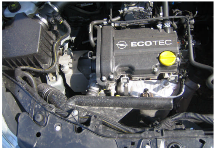
Above: A 1.4 liter twin-cam gasoline engine mated to a 5-speed manual transaxle. An amazingly compact engine, the cylinder head is only a foot long! By the way, that closed-end black plastic tube above the exhaust manifold is a Helmholtz resonator, intended to silence air cleaner drone.
