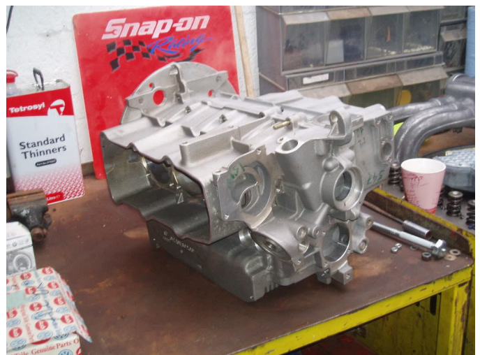
The aluminum WBX6 engine block without its cylinder barrels. The two crankcase halves are bolted together.
