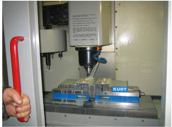
Corvair Performance Workshop. Day 1. CNC milling machine in action at Advance Racing Suspension.
