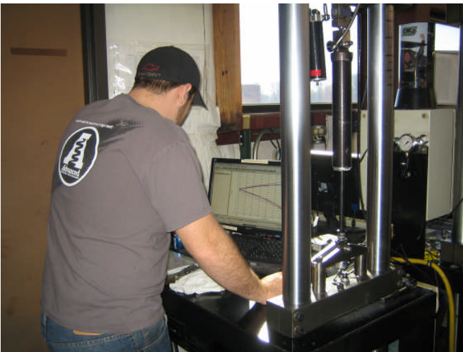
Corvair Performance Workshop. Day 1. Shock absorber going through cycle tests.
