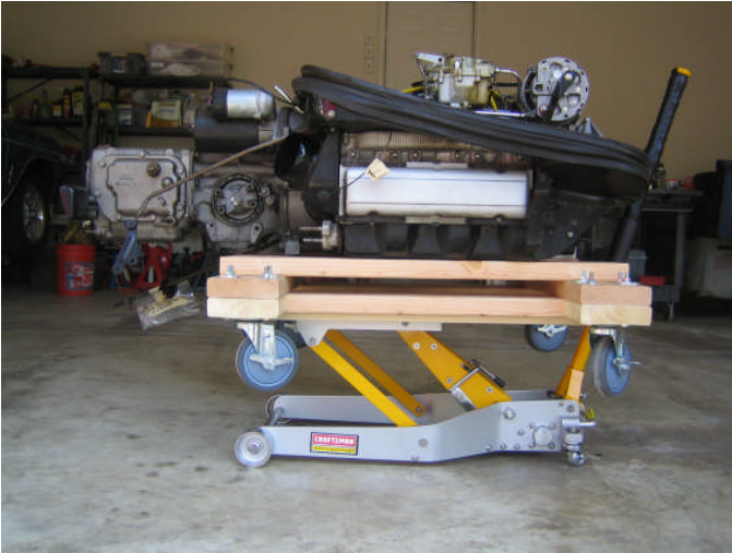
LeHeap gets a clutch job~ Corvair Unipack powertrain on Lacki's home-built engine cart.
