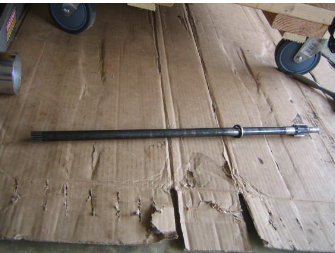
Split-ring washer fell right out of the differential snout when Lacki separated the transaxle from engine.
