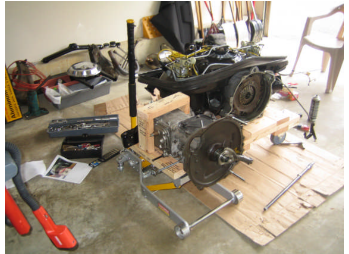
Transaxle separated from engine. Lacki used home-made alignment pins to prevent diff snout damage.
