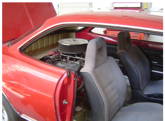
Compared to the Crown setup, Kelmark conversion provides more space for driver and passenger.
