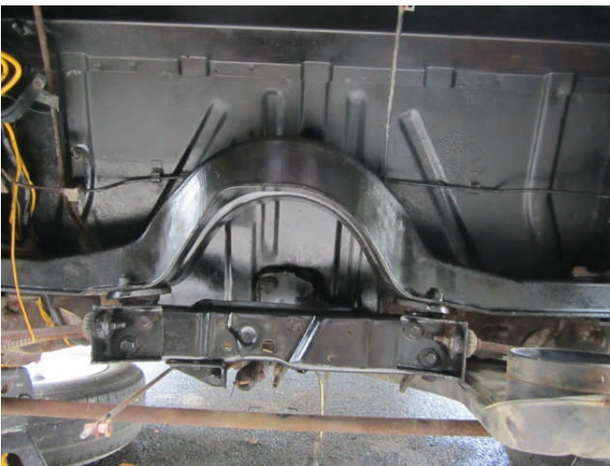
Tim repainted the entire engine compartment with POR-15. Crown anti-roll bar at bottom of photo.
