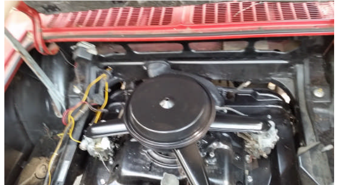
A trusty 110 engine will serve as the power plant for the time being. Tim removed and repainted all the tin.
