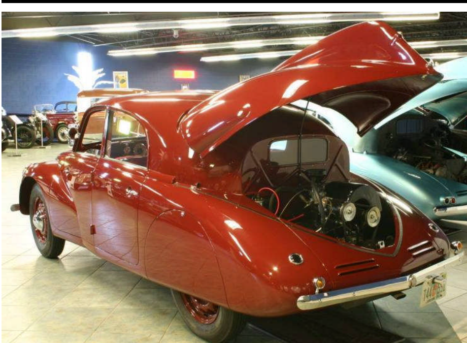
1938 Tatra T97. Little brother to the V8 Tatra streamliners, it featured a backbone chassis, swing axle suspension and rear mounted air cooled 4-cylinder boxer engine. Introduced in 1936, it was a production car that preceded the Volkswagen Beetle by several years. Photographed at the Tampa Bay Automobile Museum by Douglas Wilkinson.
